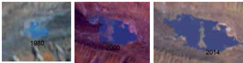
Figure 14. Growth of a moraine dammed lake in western Himalaya as shown using Landsat MSS, IRS LISS III and Landsat OLI/TIRS data of ablation season.
