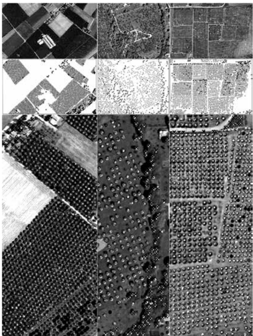
Figure 14. Illustration of the results of the tree counting for the three test images: Grenoble (left column), Briacciano (center column), and Juazeiro (right column). The empty circles represent the trees that were found, “x” represents the false positives and the black circles represent the false negatives.
