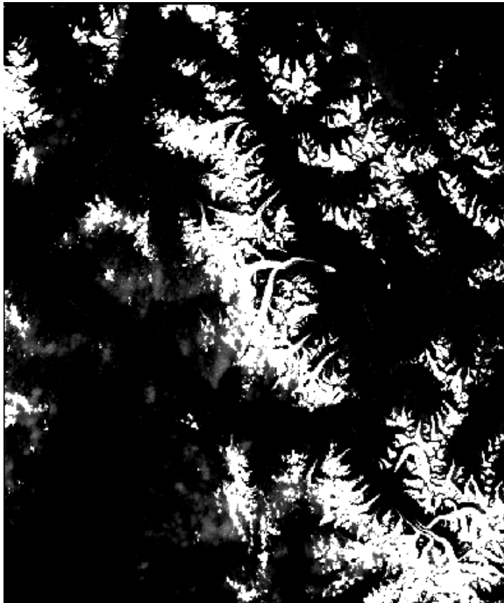
Figure 6. Glacier delineation with NDSI showing glaciated (white) and non-glaciated (black) regions, Chandra-Bhaga basin, Himachal Himalaya, India, obtained from IRS LISS III dated September 11, 2000, data.
