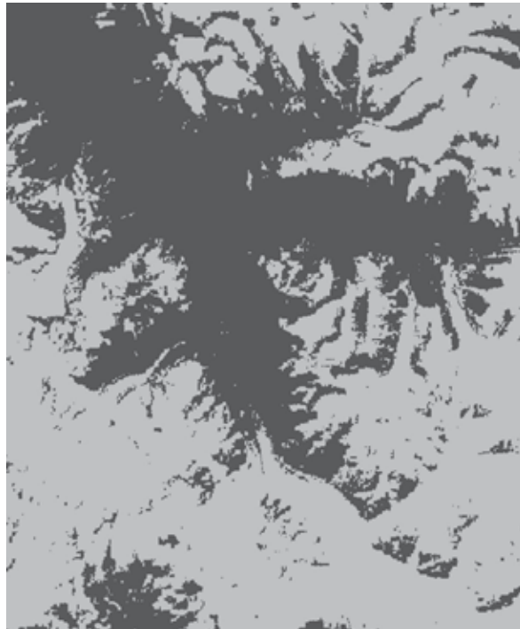
Figure 4. NDSI of Gangotri glacier derived from IRS LISS III image, September 11, 2000, for ablation season. The white part is the snow covered area and the grey is the non snow areas.
