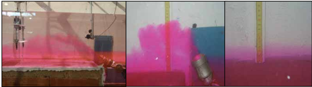
Fig. 4. Physical model test of a brine single jet discharge. Figure 4A shows the jet flow path in the near field region. Figure 4B) shows a detail of the jet orifice and flux exit. Figure 4.C) shows the brine hypersaline plume which is typical of the far field region.
