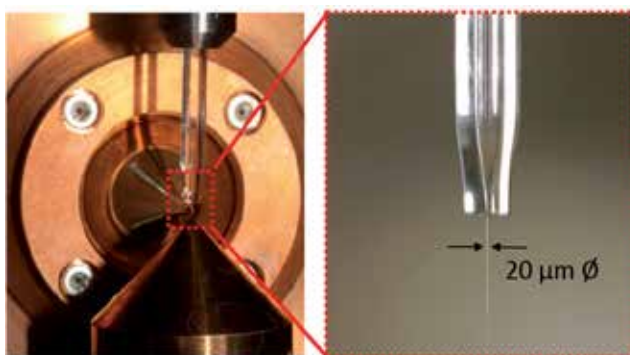
Figure 4. Micro-jet implemented for photo-electron spectroscopy. Courtesy of José Ojeda, EPFL.
