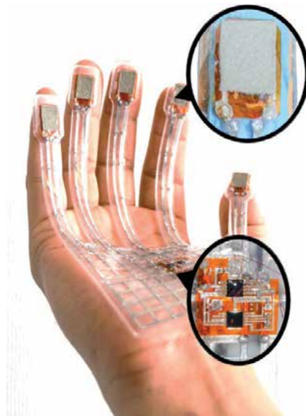
Figure 28. Photograph of the stretchable multi-point, wireless pressure sensor prototype.
