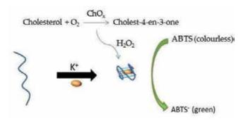
Figure 2. Schematic diagram of the G-quad-based colorimetric sensor for cholesterol.
