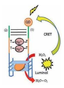
Figure 8. Detection of Hg<sup>2+</sup> through CRET from luminol that is oxidized by DNAzyme to QD.
