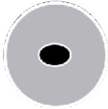
Figure 2. Fibre cross-sections with cylindrical symmetry broken by manufacturing process that leads to fibre birefringence.
