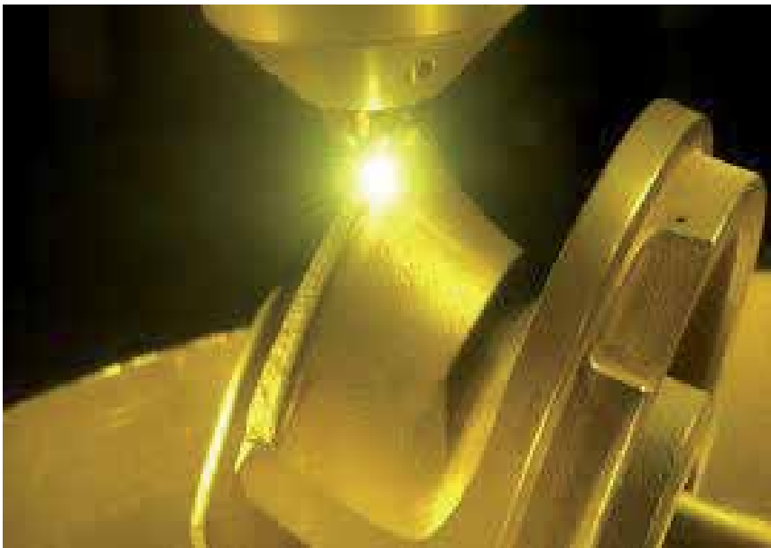
Figure 8. Fabrication of impeller pump using LENS™ [40].
