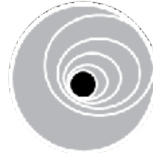
Figure 2. Fibre cross-sections with cylindrical symmetry broken by manufacturing process that leads to fibre birefringence.
