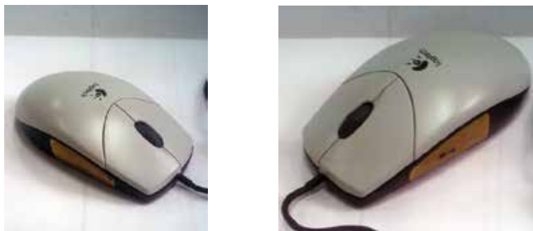
Fig. 18. Manipulator of mouse type with the built-in combined sensors: a view from the PPG sensor is shown in the left and a view from GSR and ECR sensors is shown in the right.
