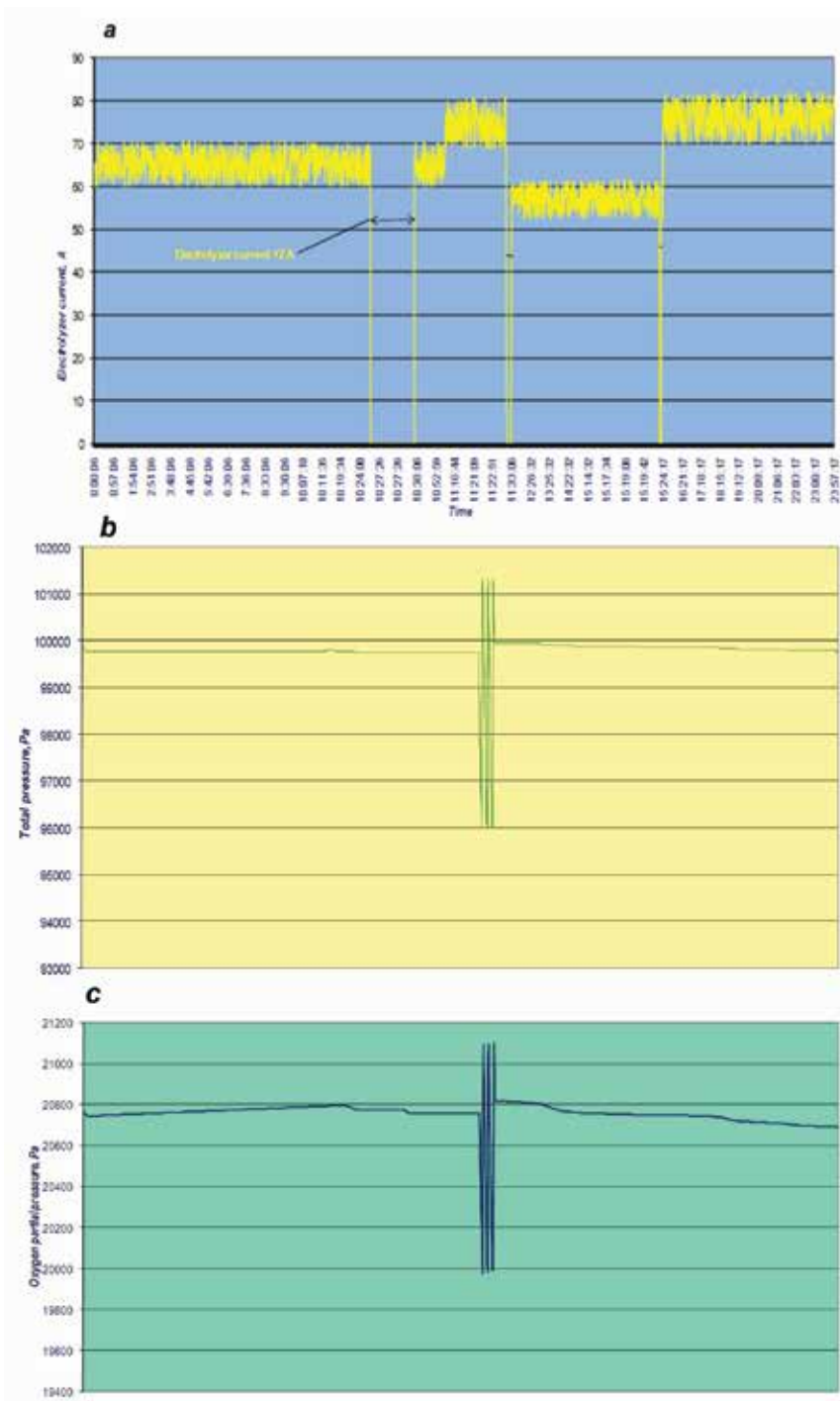
Fig. 19. Localization of the ONS 'ELECTROLYZER CURRENT < 2 A' (Crewmember 1002): a - electrolyzer current change; b - total pressure change; c - oxygen partial pressure change.
