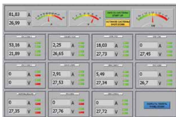
Fig. 14. Control panel of the PSS VS.
