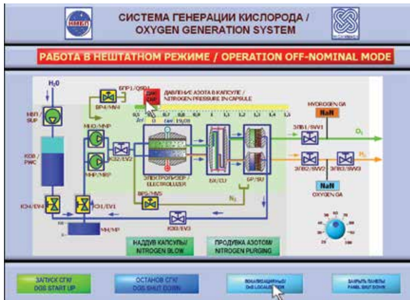
Fig. 12. Front panel of the 'OGS' virtual simulator subroutine in 'OPERATION OFF-NOMINAL MODE' (Pressure in the canister is below norm.).
