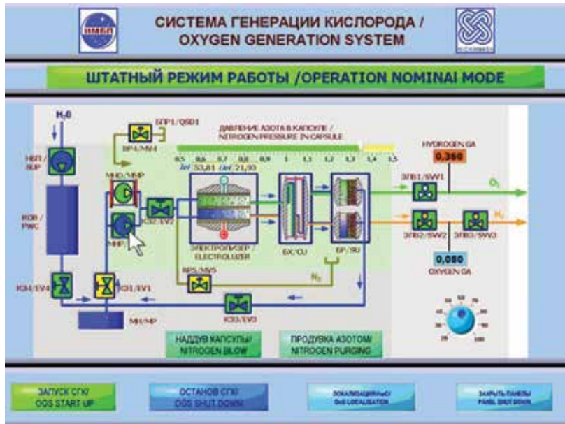
Fig. 11. Front panel of the 'OGS' virtual simulator subroutine in 'OPERATION NOMINAL MODE' (НБП/SUP=supply unit pump; КОВ/PWC=pre-purification water container; КЭИ/EVI=electromagnetic valve; МНО/MMP and МНР/RMP=main micro-pump and reserve micro-pump; БХ/CU=cooling unit; БП/SU=separator unit; GA=gas analyzer).
