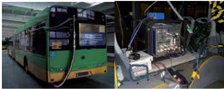
Figure 1. City bus with the measurement equipment fitted during the road tests
