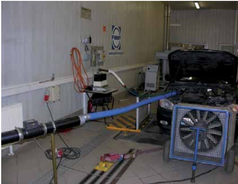
Figure 7. Photography of a test stand (visible chassis engine test stand, air supply, water vapor supply, and exhaust gas analyzer)
