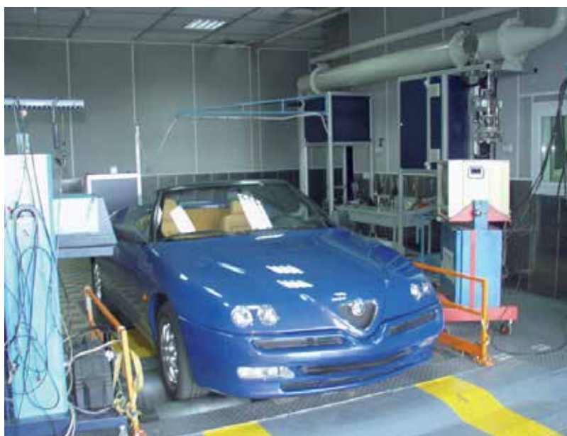
Figure 4. Chassis dynamometer SCHENCK 500GS/60 in BOSMAL Automotive Research & Development Institute
