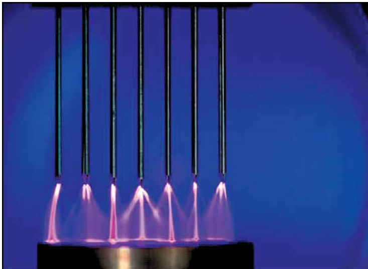
Fig. 3. b. View on a multi-tip pulsed corona discharge tested at LAPLACE-PRHE Laboratory.
