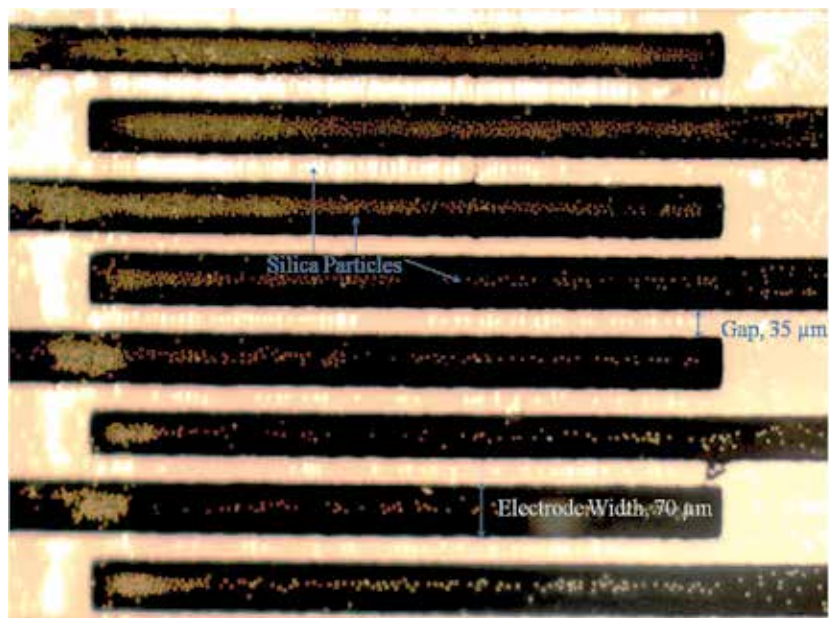
Fig. 13. Negative DEP effect on silica particles
