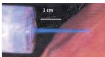
Fig. 12. Photograph of the plasma plume in contact with human skin [Reprinted with permission from (Lu&Laroussi, 2006)].
