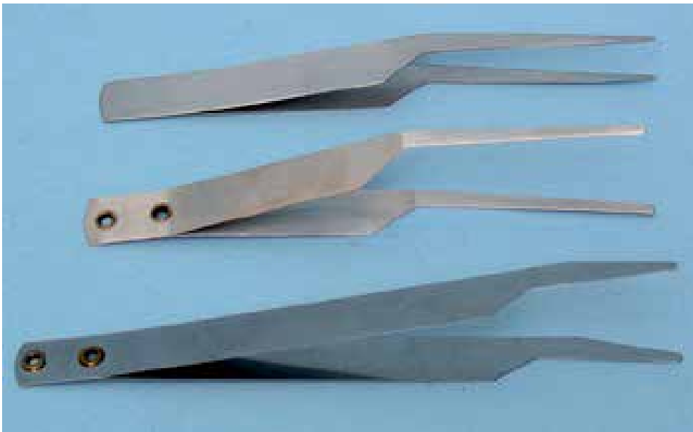
Figure 5. Storkbill (or Insect) forceps, which are made of flexible materials, aid in careful handling of samples.
