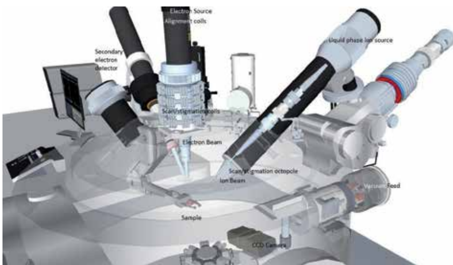
Figure 3. Construction of a dual-beam chamber
