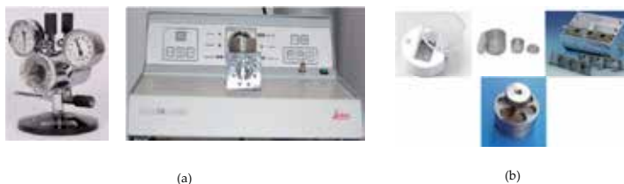
Figure 10. (a) Critical Point Dryers (CPD). The CO 2 gas cylinders are not shown. It is advisable to use a CO 2 gas of at least 99.8% purity and the gas cylinder is fitted with a siphon tube to draw liquid CO 2 from the bottom of a cylinder. (b) CPD Sample Holders, which are supplied with the CPD apparatus.
