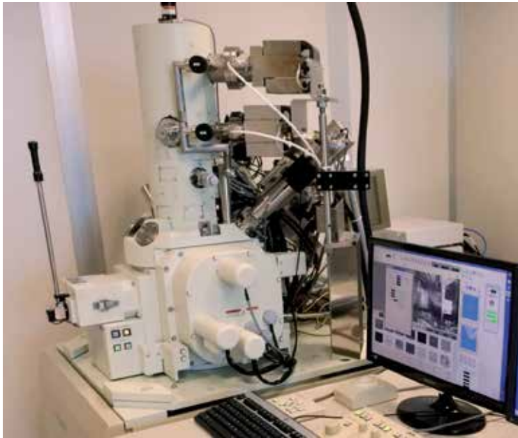
Figure 2. A commercial FIB/SEM workstation equipped with GIS, micromanipulator, and EDS detector (JEOL JIB 4601F MultiBeam System at Sabanci University Nanotechnology Research and Application Center-SUNUM)
