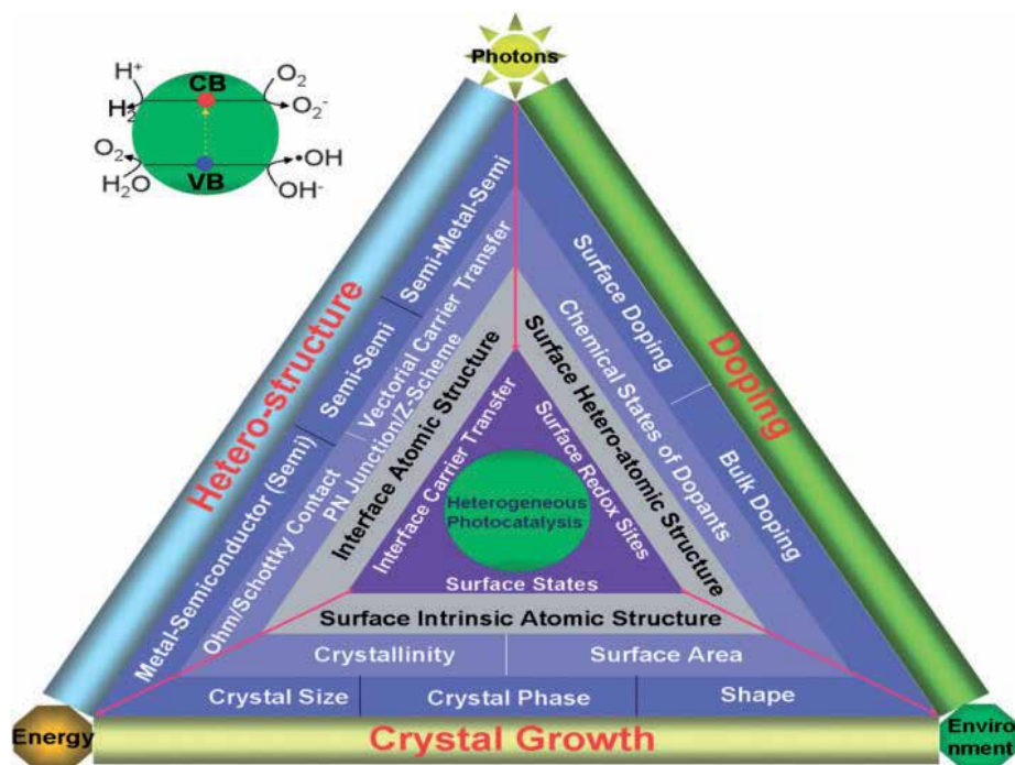
Figure 3. Correlation of key factors in crystal growth, doping and heterostructuring of semiconductors for photocatalysis. (CB: conduction band; VB: valence band) [75].
