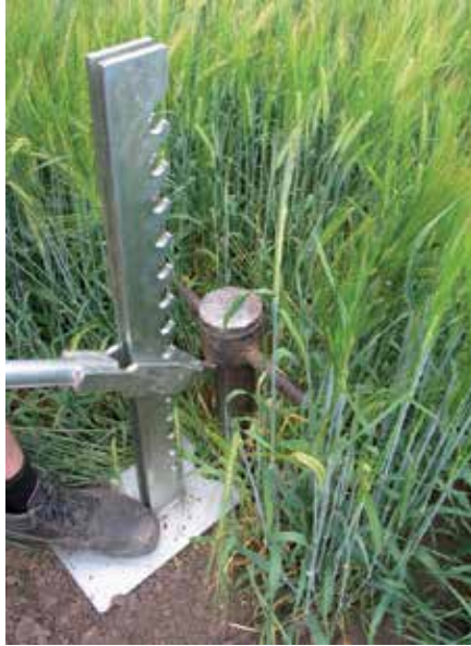
Figure 1. Sampling the root biomass for the evaluation of the relation between above and below ground parts of a plant.
