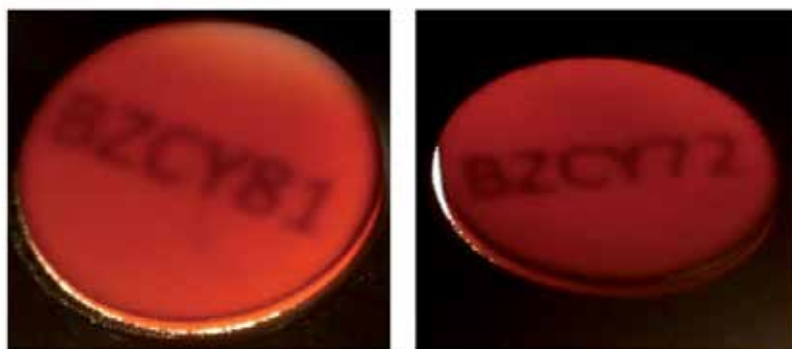
Figure 10. BZCY81 and BZCY72 specimens after NiO extraction at 1600 °C, followed by annealing in H 2 At 800 °C for 24 hrs.
