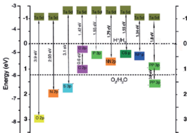
Figure 4. Band alignment of non-metal ions doped \text{NaTaO}_3 . The position of the valence band edge of pure \text{NaTaO}_3 is adopted from experiment [37].
