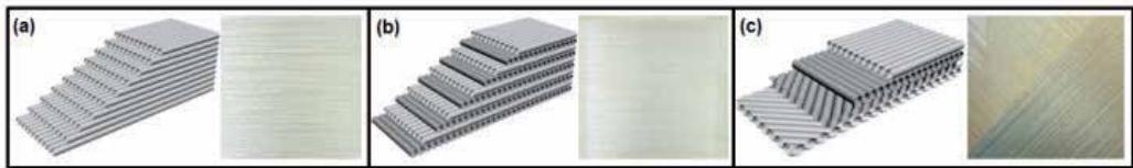
Figure 8. (a) Unidirectional non-interlaced fabric schematic and fabric (b) biaxial non-interlaced fabric schematic and fabric, and (c) multiaxis non-interlaced fabric schematic and fabric [43].
