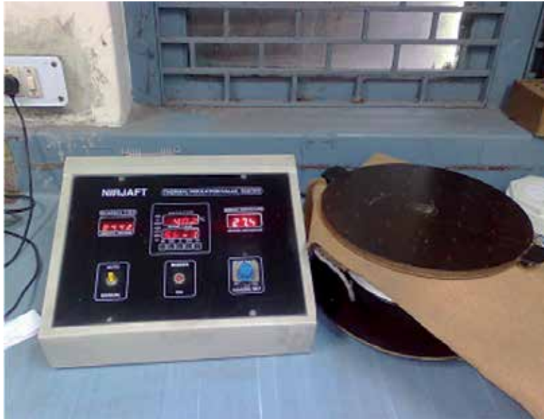
Figure 3. Instrument for measuring the thermal resistance of fabrics [19]
