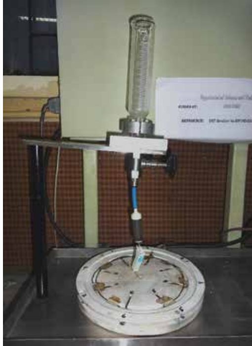
Figure 5. Photograph of the instrumental set-up for measuring in-plane wicking
