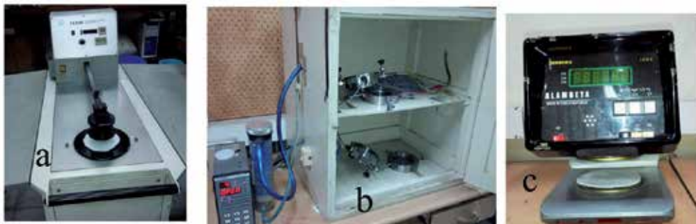
Figure 4. (a) TEXTEST air permeability tester; b) moisture vapour transmission tester (Model CS-141); c) Alambeta (Sensora) for heat transmission
