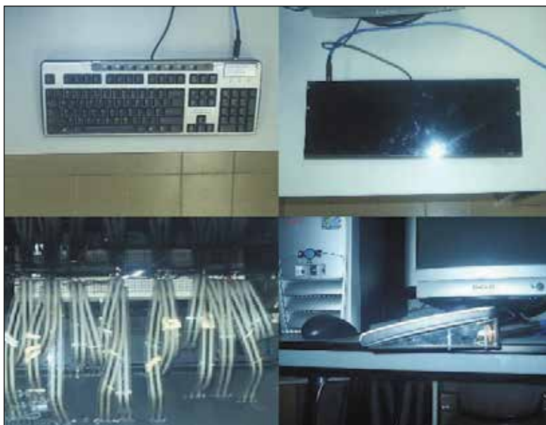
Fig. 4. Pressure sensitive alphanumeric keyboard (biokeyboard).
