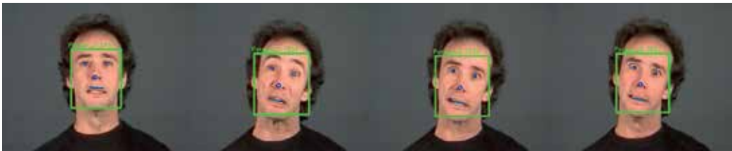
Fig. 6. Facial element detection results for a video stream extracted from the DaFEx Database.
