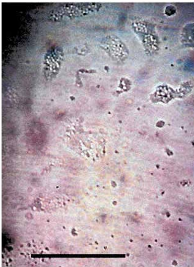
Fig. 8. Vesicle- PFNP clusters, obtained by mixing DDAB and PFNP in number ratios 300/1 and recovering the precipitates. They are visualized through a Zeiss Optical Microscope using normal light. The bar size in the bottom is 100 \mu\text{m} large.
