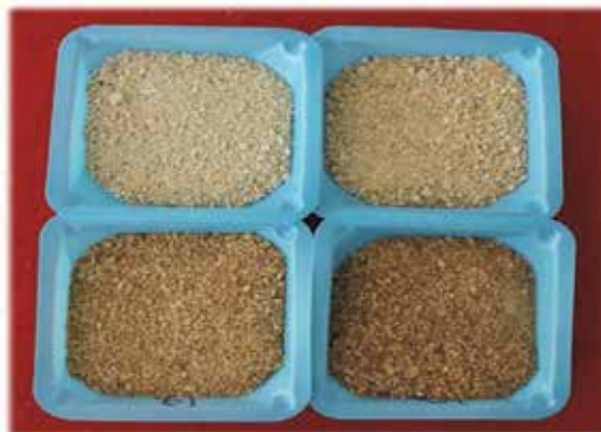
Fig. 2. Soybean meal samples exposed to varying temperatures with samples on the bottom row subjected to excessive heating as noted by the darker color (Courtesy of Dr. N. Dale, Department of Poultry Science, University of Georgia).
