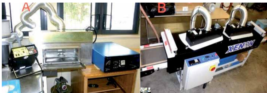
Fig. 3. A. SteriPulse XL-3000 batch PUV system; B. LHS40 continuous PUV system, as manufactured by Xenon Corporation (Wilmington, MA).
