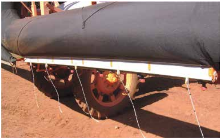
Fig. 1. “Nylon thread method” for measuring air speed in a sleeve boom sprayer.
