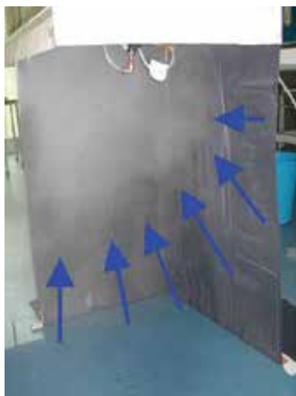
Fig. 11. Pneumatic walls supplied at 6 \cdot 10^5 Pa and 700 mm from ground
