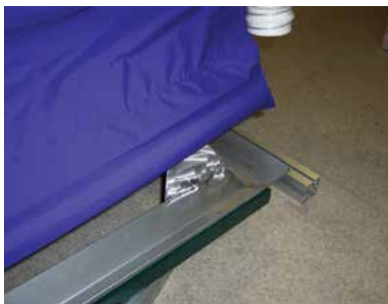
Fig. 25. Lower pneumatic sealing in DeVoPeS
