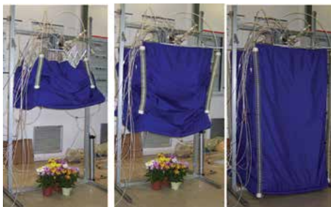
Fig. 24. Example of textile cover sheet retraction/extension in the laboratory
