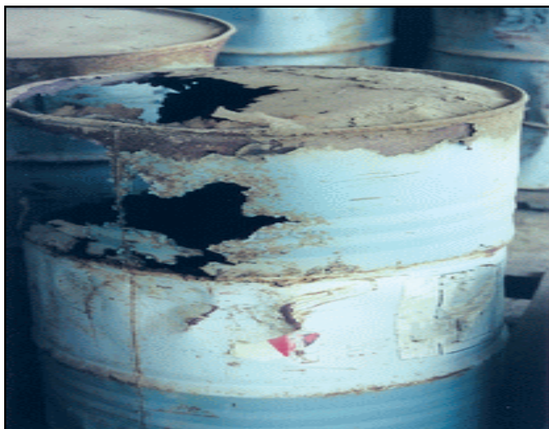
Fig. 2. Corroded pesticide container
