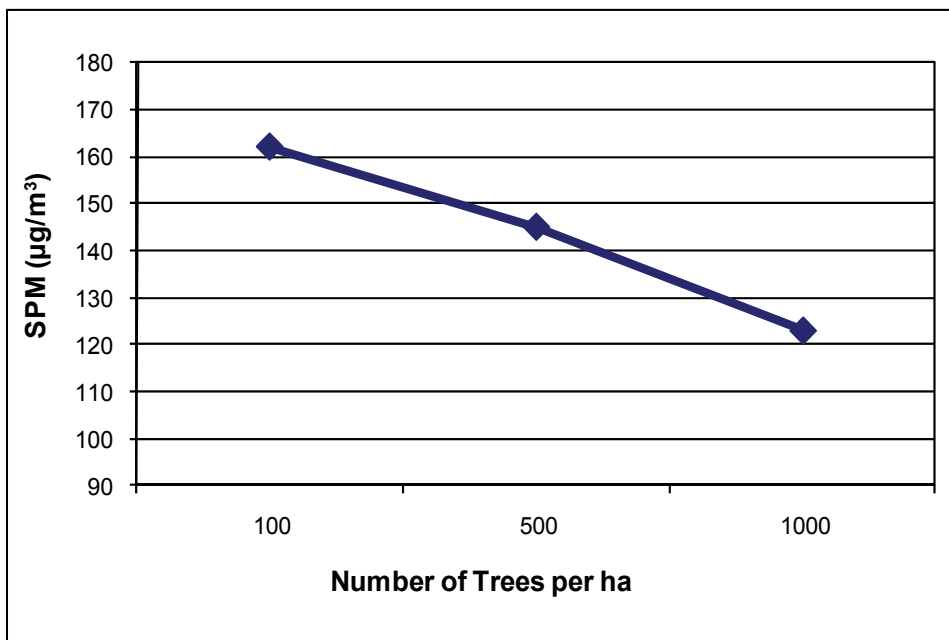
Fig. 2. Relationship between number of trees (per ha) and ambient SPM concentration (Slope: 0.04 and Intercept: 166.17)
