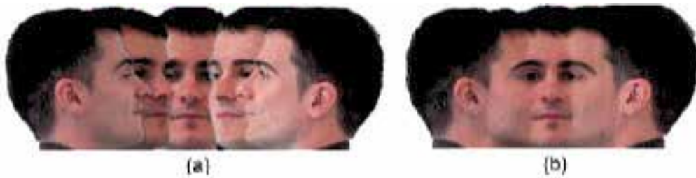
Fig. 12. (a) Set of images used for the creation of the training data; (b) Example of a 180° texture training image (Rama & Tarrés, 2007)
