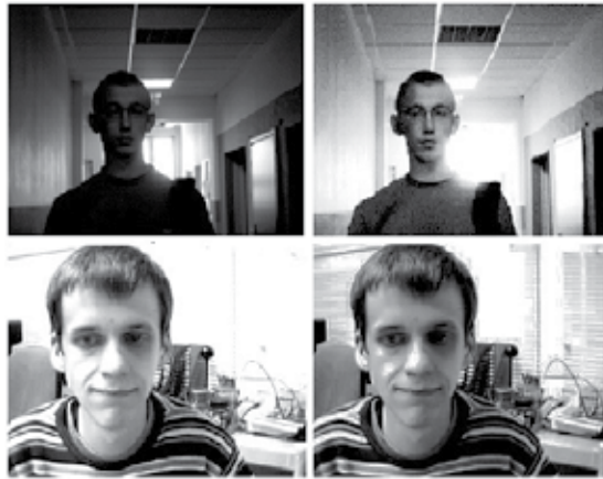
Fig. 2. Histogram equalization examples. On the left - original images, on the right - processed images. On the first image equalization significantly improves the quality of the face image, while on the latter the effect is opposite.
