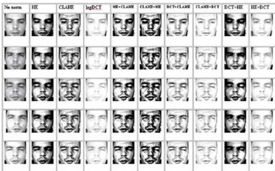
Fig. 15. Illustrative examples of various illumination normalization techniques applied to a representative subset of face data.
