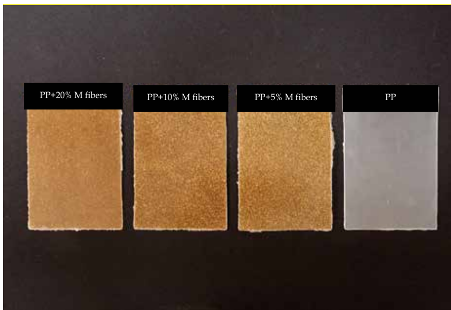
Fig. 4. Biodegradable flax composites made of polypropylene (PP) enriched with different content of bioplastic flax fibres (M plants). The control composite is made of polypropylene with no addition of flax fibres
