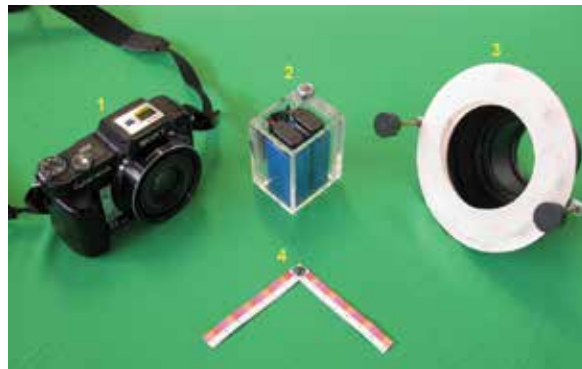
Fig. 3. Current Illuminator prototype. 1: Sony Digital Camera. 2: Illuminator power supply. 3: Illuminator. 4: Colour ruler (size, colour and focus reference)
