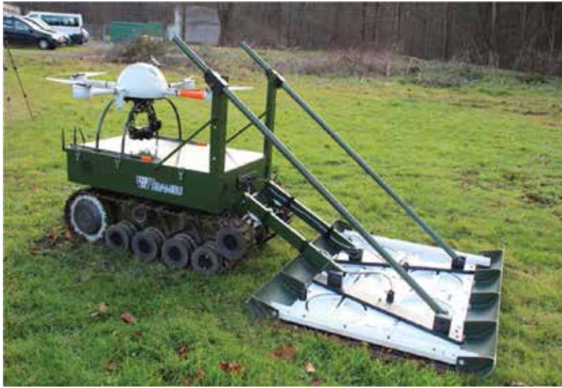
Figure 7. The teoDOR equipped with the MCMD and a TCP box positioning system.
