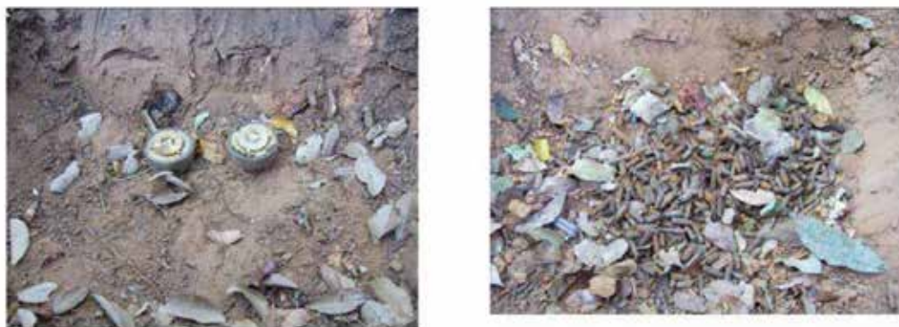
Figure 2. Some of the objects found after demining operations with metal detectors in the M7753 minefield, Province of Siem Reap, Cambodia [4].
