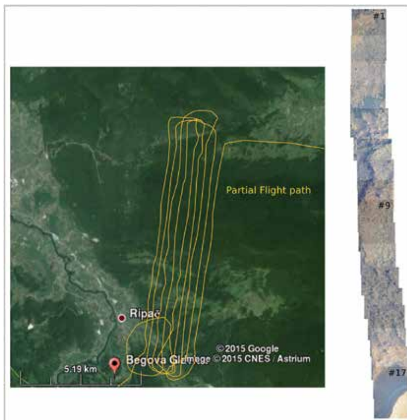
Figure 1. Example of a partial aerial campaign over Bihać region in Bosnia and Herzegovina. Left: the partial flight path. Right: a stripe made of 17 colour photographs taken during the flight.
