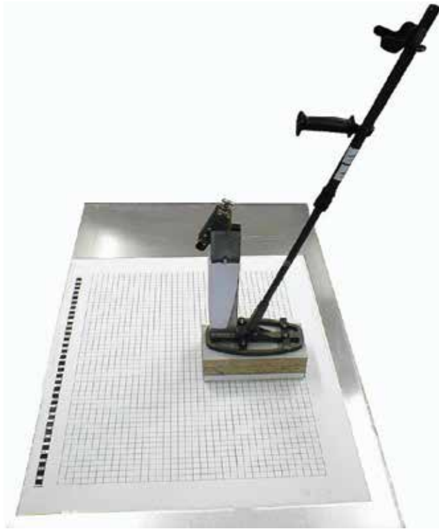
Figure 15. Evaluation grid and placement of the detector.
