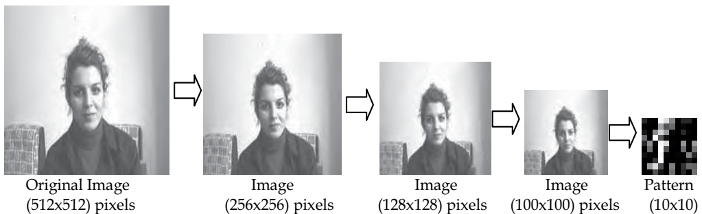
Figure 5. Image pre-processing before neural network training or testing
