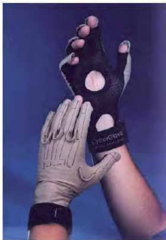
Figure 5. The 'CyberGlove' for hand gesture recognition [Bllinghurst, 2002]
