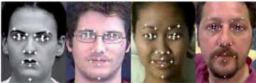
Figure 4. Examples of first-effort results of the facial point detector of Vukadinovic and Pantic (2005) for samples from (left to right): the Cohn-Kanade dataset, the MMI database (posed expressions), the MMI database (spontaneous expressions), and a cell-phone camera
