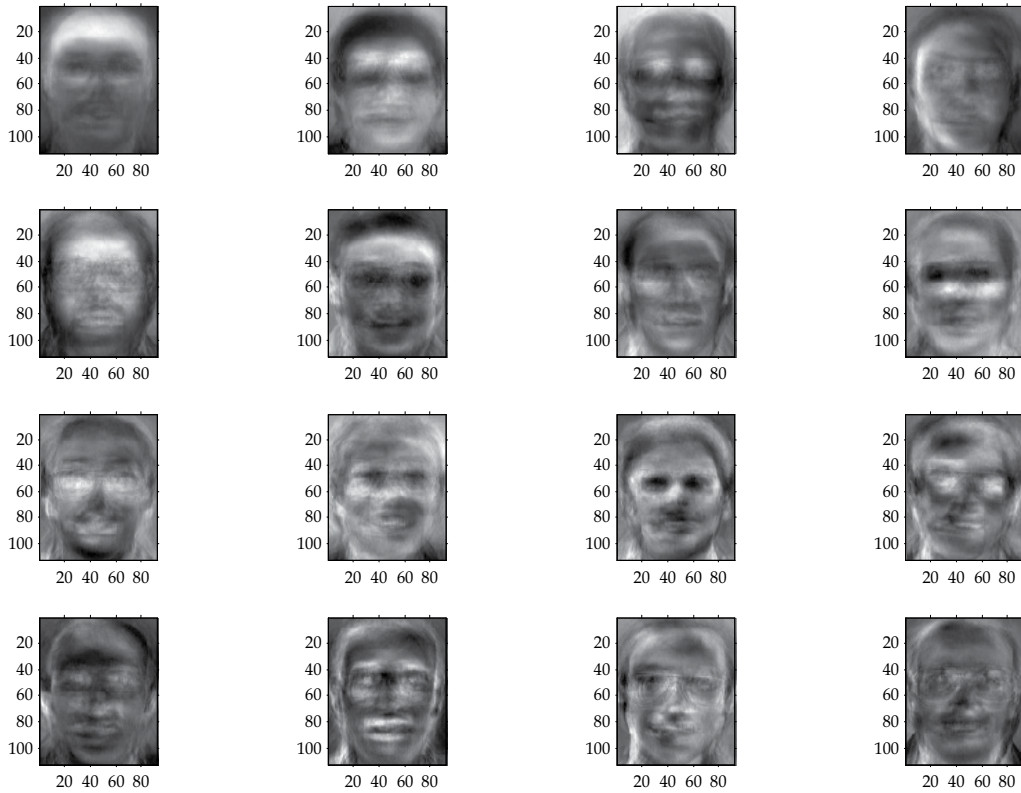
Figure 2. First 16 eigenfaces with highest eigenvalues
