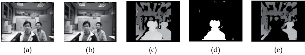
Figure 2. Extraction of a person-of-interest in a disparity image. (a) left image (b) right image (c) disparity image (d) person-of-interest (near face) (e) far face and background
