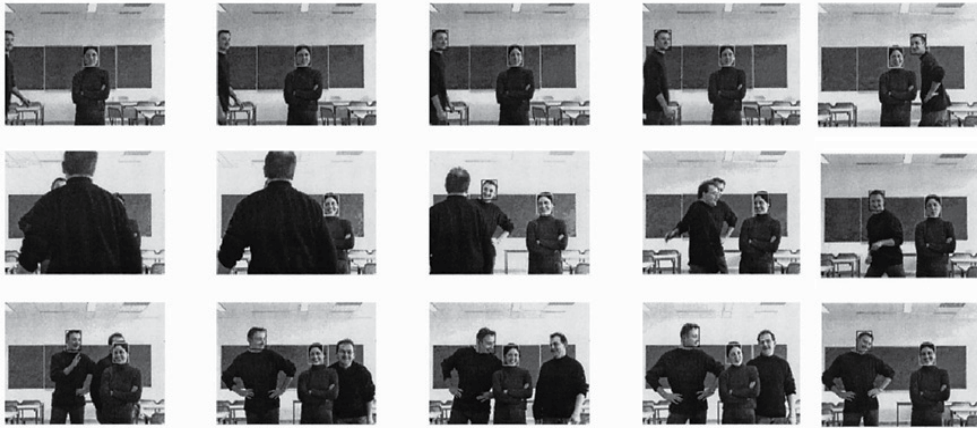
Figure 4. Some results of face tracking and identity verification
