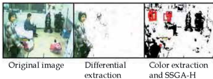
Figure 7. Human detection results from the ceiling camera of the environmental system by SSGA-H
