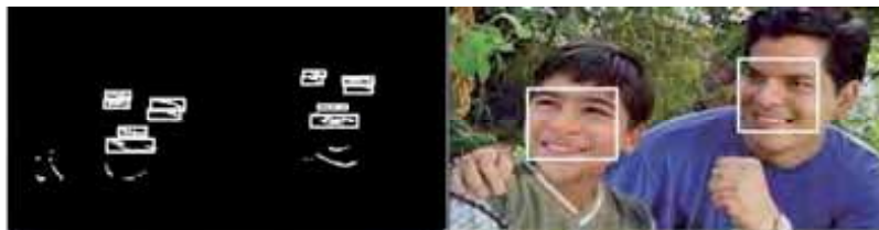
Figure 6. Results of Face Detection a) Facial Feature extraction b) Detected face in box
