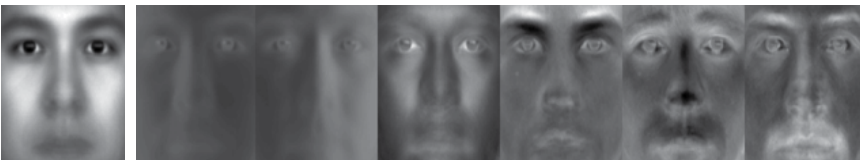
Figure 1. From left to right: PIE No-Light database mean face image followed by the first 6 Eigenfaces
