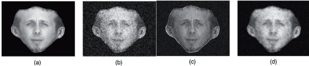
Figure 20. (a) original image, (b) original image with added Gaussian noise, (c) FFT image using the spectrum amplitude of (b) and the phase of (a) and (d) FFT image using the spectrum amplitude of (a) and the phase of (b)
