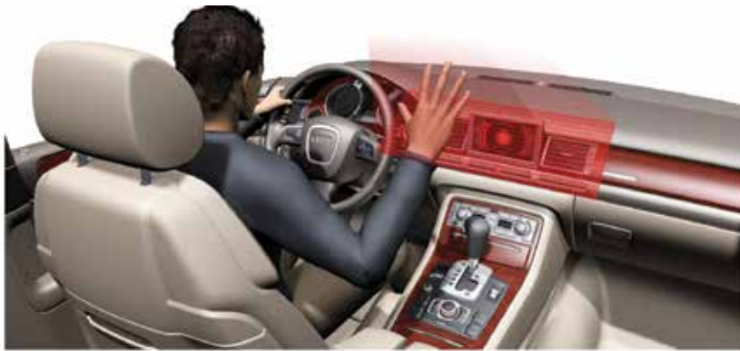
Fig. 4. Smart airbag application using a PMD TOF vision systems (Hussmann & Hess, 2006)
