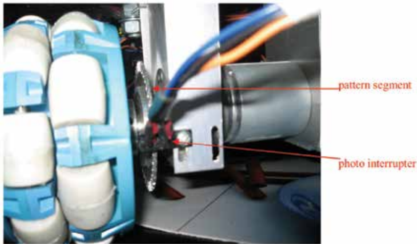
Fig. 7. The wheel encoder
