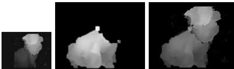
Fig. 6. (a)disparity map generated from 160x120 stereo images, (b) from 320x240 stereo images, (c)Composition of above disparity maps
