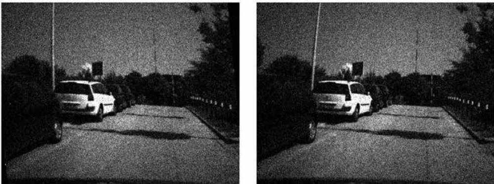
Fig. 12. A stereo pair from a perturbed 1000-frame video. The standard deviation of the added Gaussian noise is 20. The left images are synthesized using the ground-truth road parameters.
