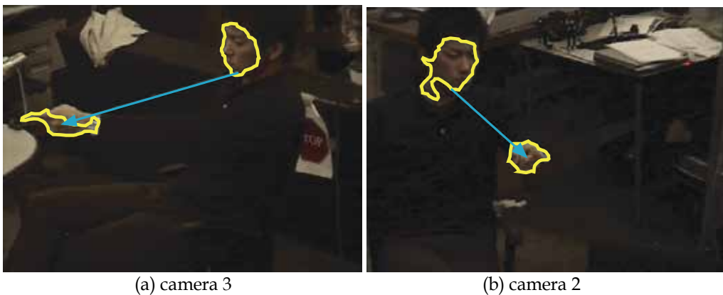
Fig. 11. Example of detected pointing using face and hand regions
