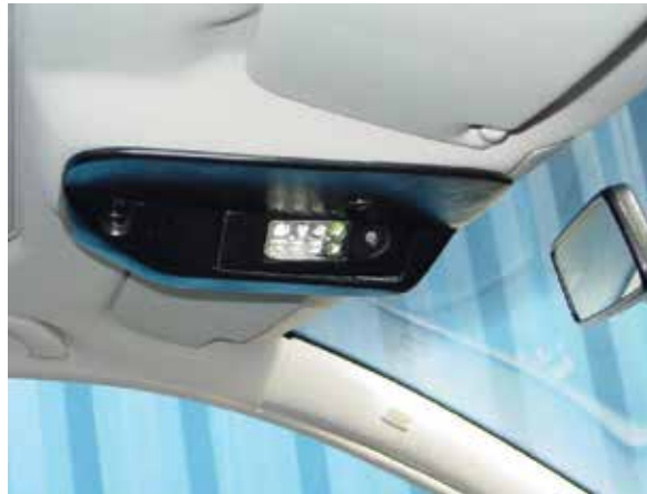
Fig. 4. Smart airbag application using a PMD TOF vision systems (Hussmann & Hess, 2006)
