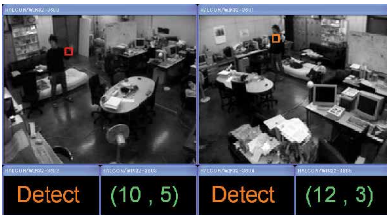
Fig. 8. Example of detected hand waving by two cameras
