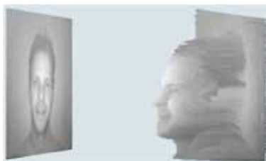
Fig. 2.7. Texture and Depth map of the SR3000 camera
