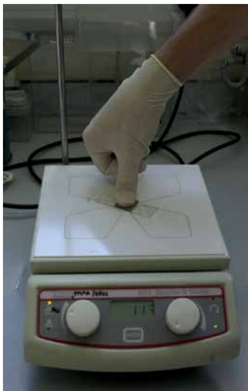
Fig. 10. A simple setup for hot embossing using a hotplate.
