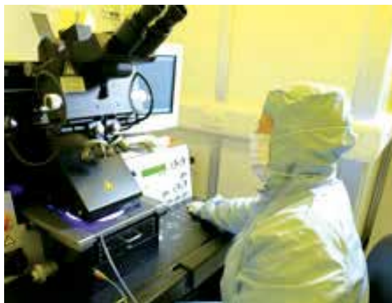
Fig. 3. The photolithographic patterning is done on a mask aligner where accurate exposure can be controlled. Image courtesy of the James Watt Nanofabrication Centre @ Glasgow
