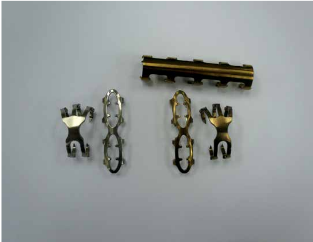
Fig. 6. Patellar concentrators and other bone concentrators with the left one showing two raw concentrators and the right one showing the three concentrators after the quasi DC-PIII treatment.
