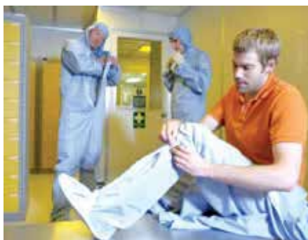
Fig. 1. Preparing for entering the clean room involves dressing in a clean room suit. The yellow light of the clean room area is visible in the background. Image courtesy of the James Watt Nanofabrication Centre @ Glasgow
