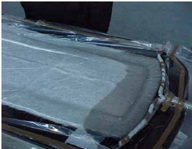
Fig. 45. Resin injection process
