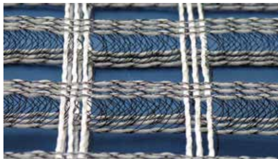
Fig. 23. Net spacer used for textile reinforced concrete
