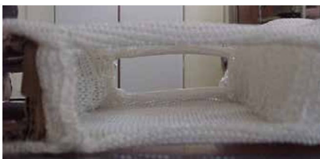
Fig. 24. Sandwich fabric with connecting knitted layers
