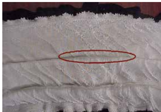
Fig. 37. Preform with jersey evolution on selected needles
