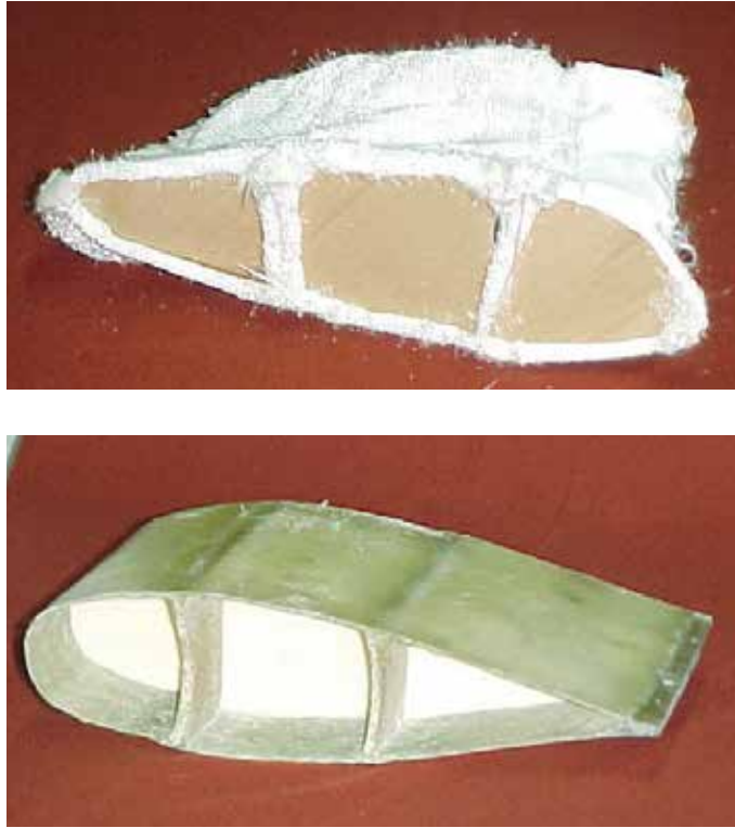
Fig. 46. Composite wing – aspect before and after resin injection
