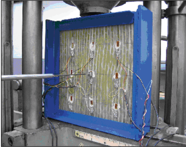
Fig. 17.5. Test rig and imperfect composite plate
