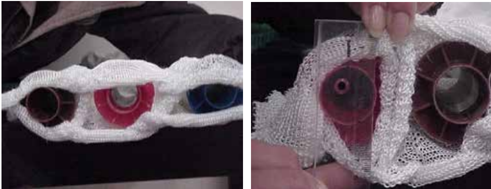
Fig. 39. Connection layers – cross section view and aspect of the first connection layer
