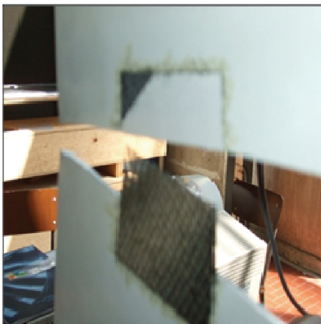
Fig. 6. The crack propagated in the adhesive layer that leads to the sliding of the full patch The configurations B demonstrate again the role of the curing procedure and a small variation in the SIF provided a larger difference in the fatigue life.
