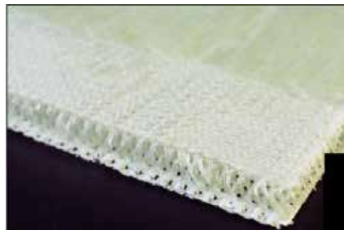
Fig. 22. Spacer fabric made of glass fibre
