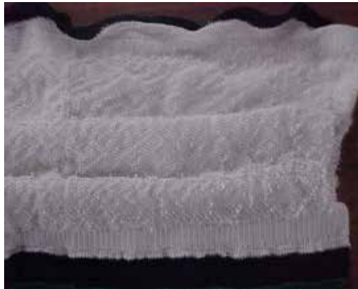
Fig. 38. Preform with jersey evolution on selected needles and fleece in-lays
