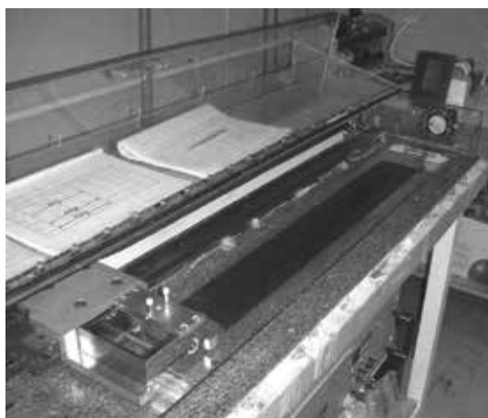
Fig. 9. Picture of discontinuous tape caster in SPCTS lab of Limoges, France.
