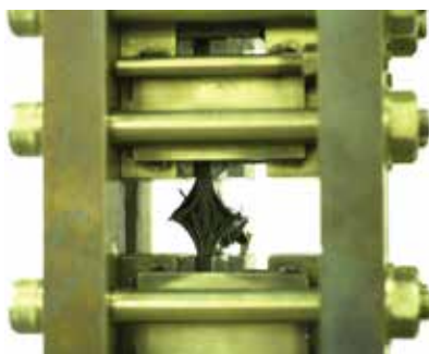
Fig. 8. External view of static compressive failure of an NH specimen at RT
