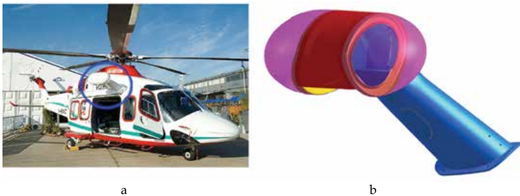
Fig. 2. a) winch arm mounted on the helicopter, b) 3D model of winch arm
