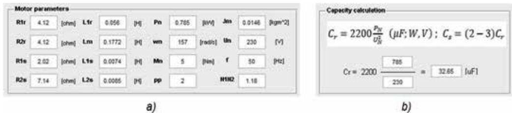
Figure 10. (a) The panel for input and changes basic parameters of the motor. (b) The panel for calculation of value of the capacitor connected into the auxiliary phase.
