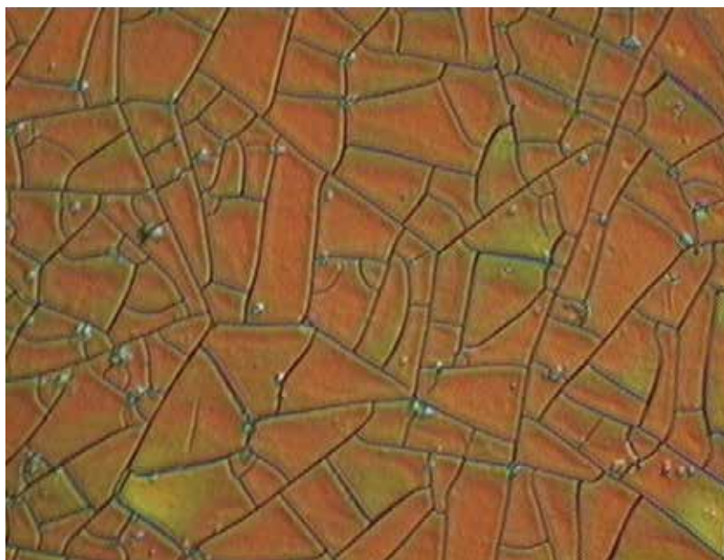
Figure 2. Optical Micrograph of an electrodeposited cerium oxide film on stainless steel. 800x magnification. (from T. Golden).
