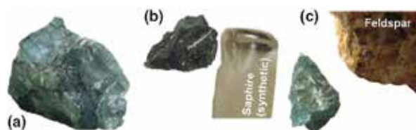
Fig. 14. Specimen of apatite from Sljudjanka, Bajkal (a) shows white color of scratch (b). The sample can be also scratched by minerals with hardness \geq 6 (feldspar and higher) on the Mohs scale (c).
