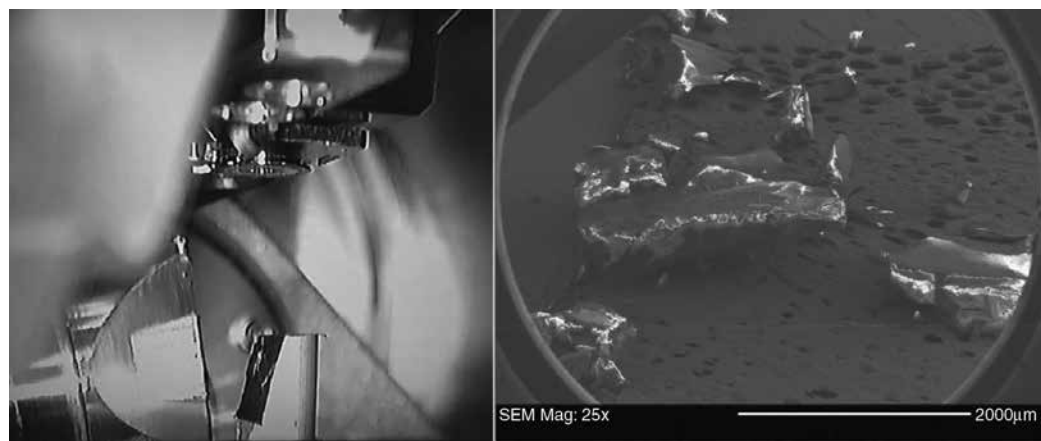
Fig. 22. Sample stage (a) and microphotograph of fluorapatite fragments used for EBDS (b).
