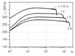
Fig. 34. Cyclic deformation curves at 300°C
