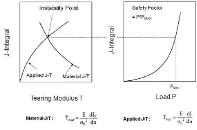
Fig. 9. Graphical illustration of J/T method
