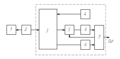
Fig. 14. Intelligent pressure OFS 1 – FFPI; 2 – optical cable; 3 – optical coupler; 4 –light emitting diode; 5 –TSOF; 6 –photodiode; 7 – microcontroller
