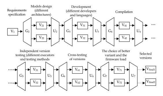
Fig. 6. FPGA-system multi-version life cycle
