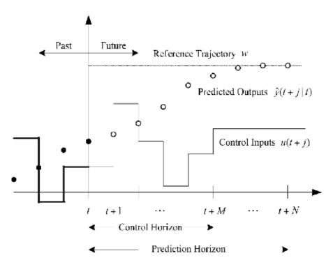
Fig. 4. Basic concept of a model predictive control method
