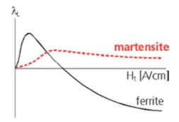
Fig. 3. Lengthwise magnetostriction and influence of microstructure
