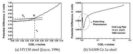
Fig. 4. Potential rise versus crack opening displacement
