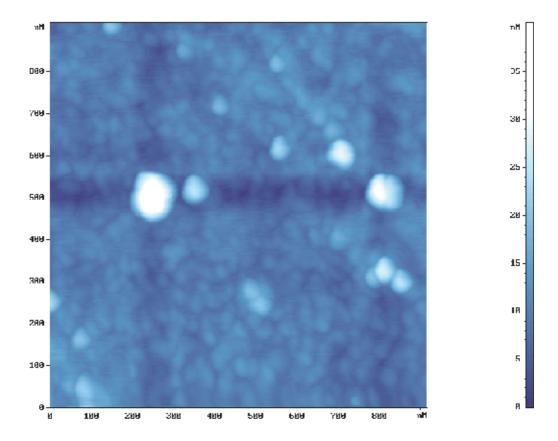
Fig. 10. Microscopic view of optical fiber tip with TiO<sub>2</sub> magnetron sputtering With processing by TiCl<sub>4</sub> steams the reaction on the surface proceeds as follows:
