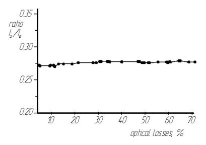
Fig. 20. Normalized output signal of the pressure OFS
