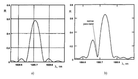
Fig. 17. Reflection spectra of strain FBG optical fiber sensor a)– without discontinuity b) – with discontinuity
