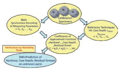
Fig. 12. The 3MA-calibration
