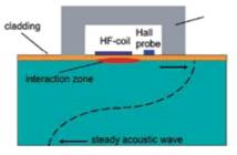
Fig. 38. Magnetostrictively excited standing wave in the PV-wall
