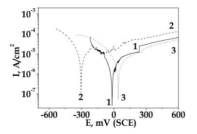
Fig. 5. PD polarization curves of HAS at 35 °C in: 1 – MCM; 2 – MCM with 10  $\mu$ g/L Cl-; 3 – MCM with 10  $\mu$ g/L Cl- and 2 mg/L MEA.
