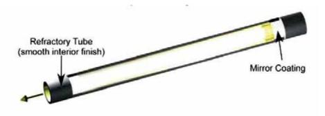
Fig. 9. Hollow-Core Light Guide Concept.
