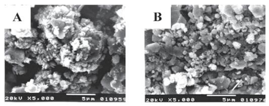
Fig. 11. SEM images of corrosion products: A – without MEA in the medium; B – in the presence of 2 mg/l MEA.
