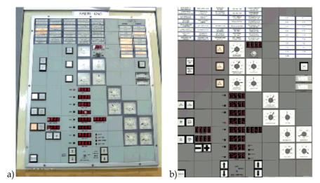
Fig. 8. a) Partial view of the real control desk; b) The corresponding virtual model.
