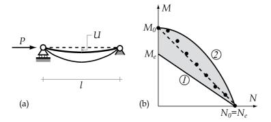
Fig. 5. Compressed column with initial imperfection
