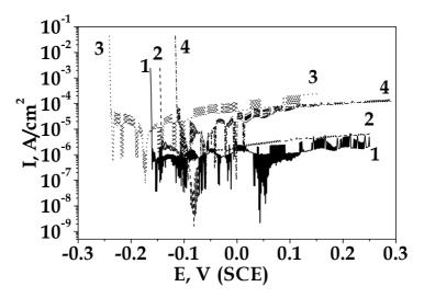
Fig. 8. PD curves of HAS in MCM with 1 mg/L Cl-, 1 mg/L SO<sub>4</sub><sup>2-</sup> and 5  $\mu$ g/L Cu<sub>total</sub>: 1 – in crack 0,5 mm at 35 °C; 3 - in crack 0,1 mm at 35 °C; 2 - in crack 0,5 mm at 95 °C; 4 - in crack 0,1 mm at 95 °C.
