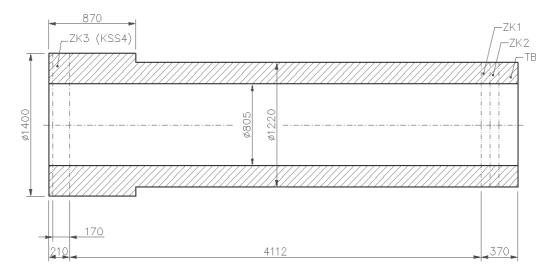
Fig. 1. Dimensions of the collector body after rough machining
