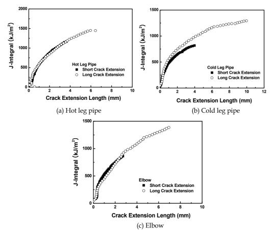
Fig. 12. The comparison of dynamic J-R curve by normalization method between the tests for short and long crack extension
