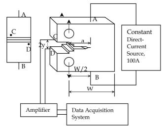
Fig. 3. Specimen geometry for dynamic J-R curve testing
