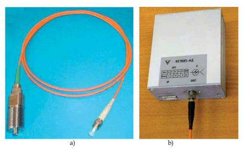
Fig. 18. General view of intelligent pressure OFS a)– sensing element (b)- optoelectronic transceiver
