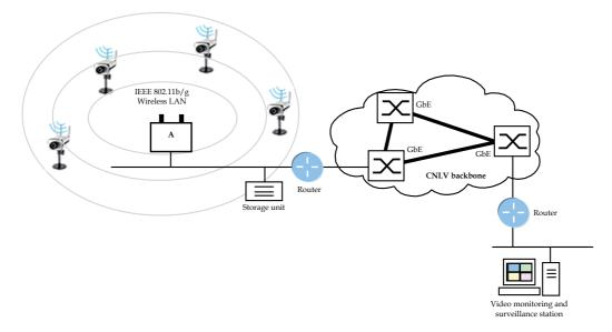
Fig. 4. Proposed wireless IP video system for the CNLV nuclear plant, Mexico.
