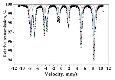
Fig. 12. Moessbauer spectra of CPs taken from SGs (average results)
