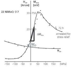
Fig. 8. Barkhausen noise peak maximum and peak separation as function of mechanical stress and stress sensitivity  $\Delta M_{Max} / \Delta \sigma$  of the German pressure vessel steel 22 NiMoCr 37 after welding and 72h stress relief annealing
