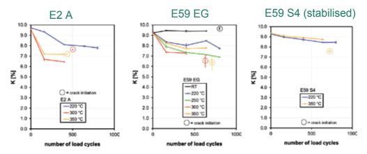
Fig. 21. Distortion factor K as function of cycle number measured after well defined fatigue intervals in test interruptions followed by a further fatiguing of the same specimen
