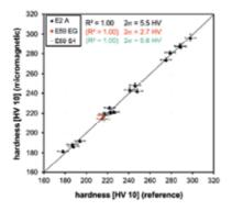
Fig. 23. 3MA prediction of the Vickers hardness 10
