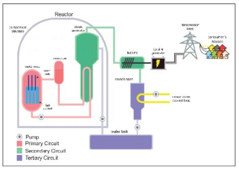
Fig. 1. PWR NPP simplified diagram<sup>1</sup>.
