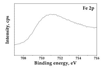
Fig. 14. XPS measurements for Fe2p from the CPs of the SGs (average results)
