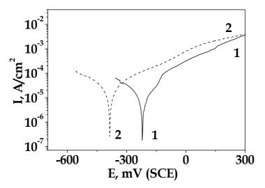
Fig. 1. PD polarization curves of LAS at 35 °C in: 1 – MCM; 2 – MCM with addition of 10  $\mu$ g/L Cl-.
