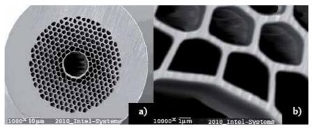
Fig. 8. Structure of the hollow core PCF at 1000<sup>x</sup> and 10000<sup>x</sup> magnifying in a microscope.
