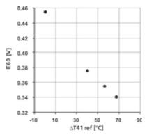
Fig. 40. Correlation of the quantity E60 with the DBTT shift at 41J Charpy energy
