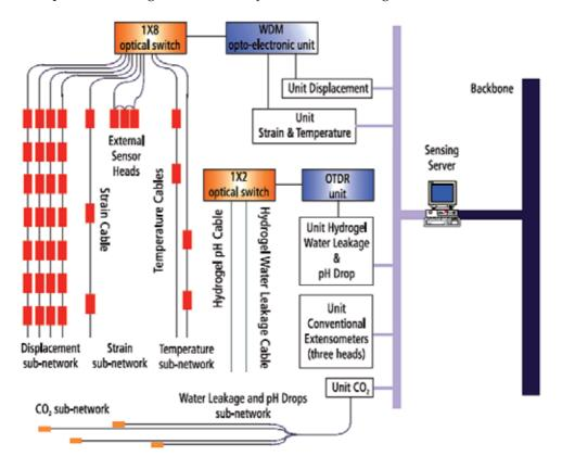
The complete circuit diagram of the OFS system is shown on fig. 23.
