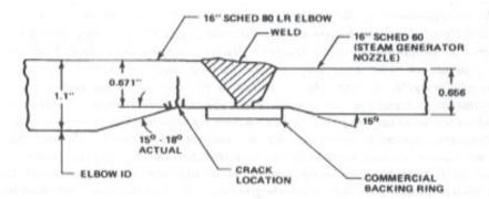
Fig. 1. Location of Cracks in PWR Feed water Pipe to Nozzle Attachment Region<sup>[1]</sup>
