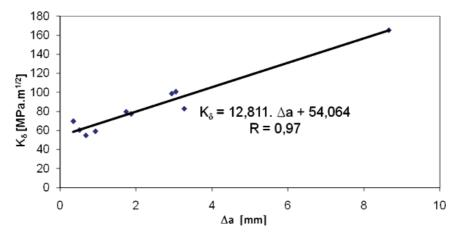
Fig. 10. The variation of  $K_{\delta}$  with crack advance  $\Delta a$  (initial  $O_2 = 4.5$  ppm, stroke rate  $1.8.10^{-6}$  mm/s).
