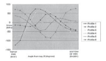
Fig. 6. Stress Distribution across Pipe Diameter for Profiles 1 through 6<sup>[4]</sup>
