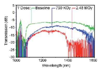
Fig. 7. Spectral transmission for 20% Ge doped silica optical fiber
