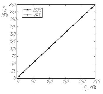
Fig. 21. Calibration characteristics of the temperature insensitive OFS
