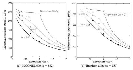
Fig. 9. Formula (21) vs computed results (dots). A defined by equation (6)
