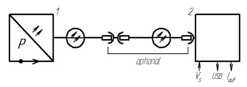
Fig. 3. Concept of remote pressure measurements 1 – OFS; 2 – optoelectronic transceiver
