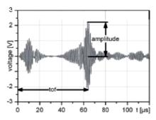
Fig. 30. Time-of-flight (tof) measurement procedure
