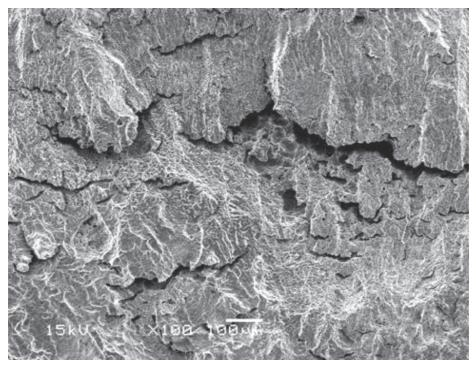
Fig. 7. Morphology of the fracture surface of the test specimen tested in water environment at 260°C (initial O<sub>2</sub> = 4, 5 ppm, R.A. = 12, 4%)
