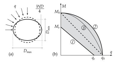
Fig. 8. Interaction domain for the tube cross section
