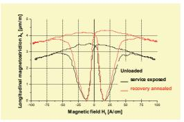
Fig. 14. The lengthwise magnetostriction of the microstructure states of Fig. 13
