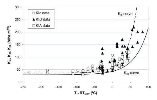
Fig. 6. ASME curves with the experimental data set used for their definition
