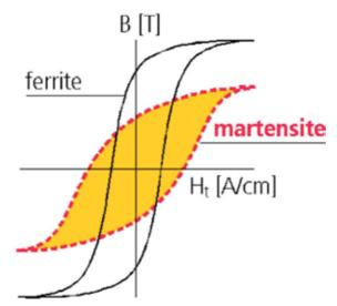
Fig. 1. Hysteresis loop and influence of microstructure
