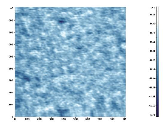
Fig. 11. Microscopic view of fiber tip with TiO<sub>2</sub> molecular layered nano-coating
