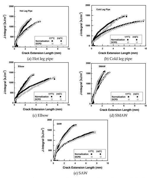
Fig. 6. Comparison of dynamic J-R curve between DCPD and normalization method when testing until load line displacement of 10mm
