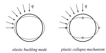
Fig. 3. Failure modalities for a long tube
