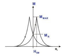
Fig. 7. Magnetic Barkhausen noise profile curve
