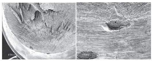
Fig. 9. Fracture surface of the test specimen tested in water environment at 260°C (initial  $O_2 = 4.5$  ppm, R.A. = 12,4%)
