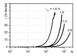
Fig. 32. Cyclic deformation curves at ambient temperature
