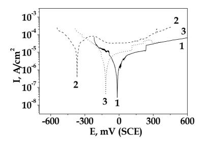
Fig. 6. PD polarization curves of HAS at 35 °C in: 1 – MCM; 2 – MCM with 300  $\mu$ g/L SO<sub>4</sub><sup>2-</sup>; 3 – MCM with 300  $\mu$ g/L SO<sub>4</sub><sup>2-</sup> and 2 mg/L MEA.
