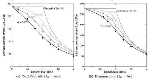
Fig. 7. Formula (17) vs computed results (dots). A defined by equation (14)
