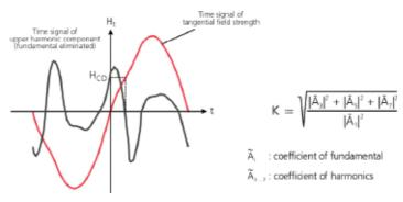
Fig. 5. Fourier analysis of the magnetic tangential field
