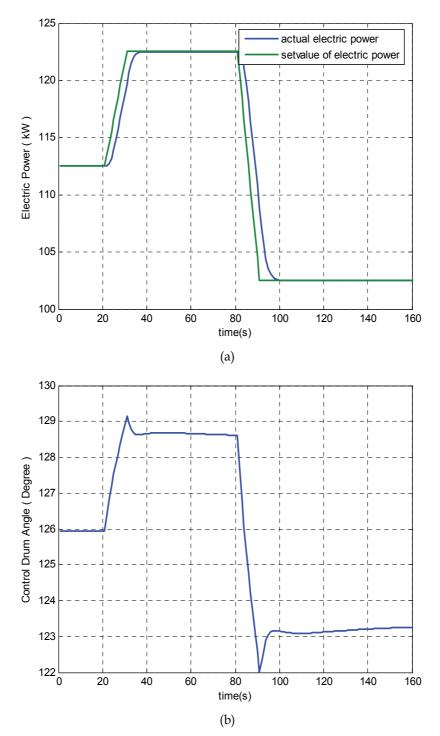
Fig. 6. (a) Electric power (TE) set point profile and the controller performance. (b) Controller response (i.e., reactivity control) in terms of the drum angle
