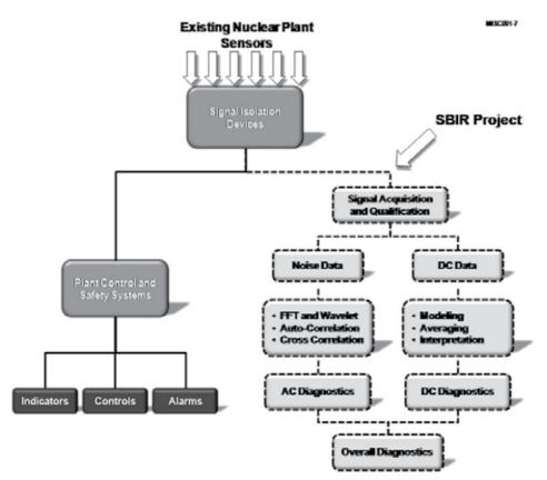
Fig. 2. Data Acquisition Signal Path for OLM
