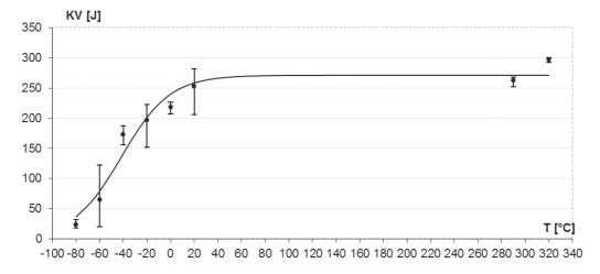
Fig. 4. Temperature dependence of impact fracture energy in the temperature range from -80  $^\circ C$  to 320  $^\circ$
