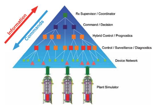
Fig. 1. Supervisory control architecture for multi-modular nuclear power plants
