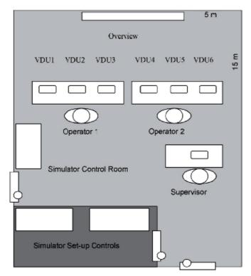
Fig. 4. LABIHS simulator room's layout.
