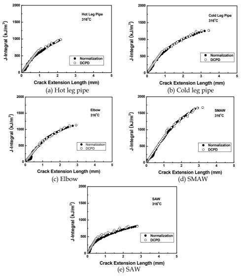
Fig. 5. Comparison of dynamic J-R curve between DCPD and normalization method when testing in accordance with crack extension criteria of normalization method
