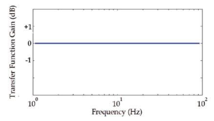
Fig. 6. Transfer gain-frequency function of a pressure optical fiber sensing system
