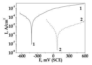
Fig. 7. PD polarization curves of HAS at 35 °C in: 1 – MCM with 1 mg/L Cl<sup>-</sup>, 1 mg/L SO<sub>4</sub><sup>2-</sup> and 5  $\mu$ g/L Cu<sub>total</sub>; 2 – MCM with 1 mg/L Cl<sup>-</sup>, 1 mg/L SO<sub>4</sub><sup>2-</sup>, 5  $\mu$ g/L Cu<sub>total</sub> and 2 mg/L MEA.
