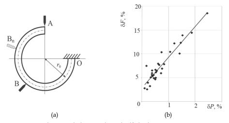
Fig. 1. Pressure sensor device with the metrological self-check (a)Location of the points of the Bourdon tube displacement measurement (b)Relationship between the relative variation of the diagnostic parameter ( $\delta F$ ) and relative error  $\delta P$  of pressure measurement
