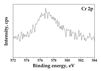
Fig. 16. XPS measurements for Cr2p from the CPs of the SGs (average results)
