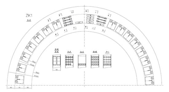
Fig. 2. Orientation of the test specimens in the testing block
