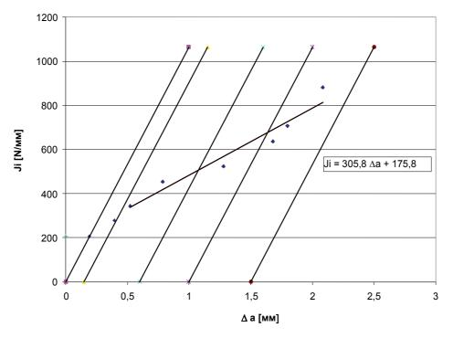
Fig. 6. J-R curve of the studied steel at 290°C determined by multiple test specimen method
