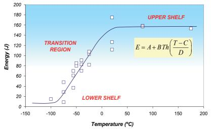
Fig. 2. Influence of temperature on the results (absorbed energy) of the Charpy test; the data were fitted to a hyperbolic tangent curve
