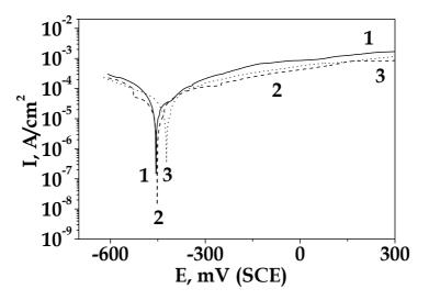
Fig. 2. PD polarization curves of LAS at 35 °C in: 1 – MCM with 300 μg/L Cl<sup>-</sup>; 2 – MCM with 300 μg/L Cl<sup>-</sup> and 2 mg/L MEA; 3 – MCM with 1 mg/L Cl<sup>-</sup> and 2 mg/L MEA.
