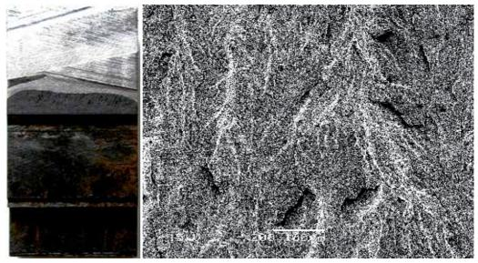
Fig. 11. Morphology of the fracture surface created by SCC, t = 260°C,  $O_2$  = 4,5 ppm,  $v_{cor}$  = 3,7.10<sup>-5</sup> mm/s
