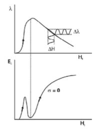
Fig. 11. Dynamic or incremental magnetostriction
