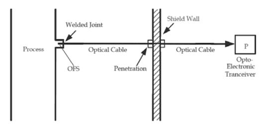
Fig. 5. New advanced structure of the pressure sensing line inside a nuclear reactor containment
