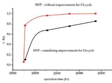
Fig. 7. Comparison of the curves of SWP failure probability with improvements and without improvements to the C4 cycle
