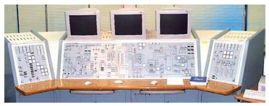
Fig. 2. Reduced-scale full-scope NPP simulator<sup>2</sup>.
