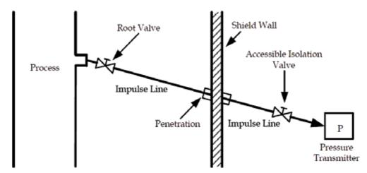
Fig. 1. Typical pressure sensing (instrument) line inside a nuclear reactor containment.
