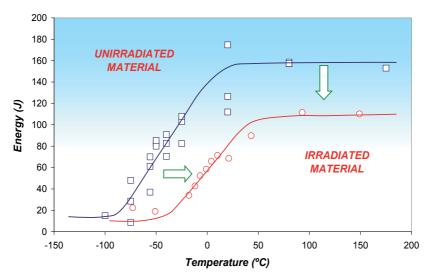
Fig. 3. Description of the influence of neutron irradiation on the Charpy curves (absorbed energy vs. temperature)
