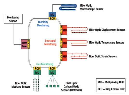
Fig. 24. All-fiber optic sensors network for SNF repository
