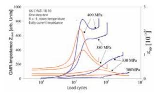
Fig. 27. One-step stress controlled fatigue tests at room temperature
