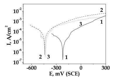
Fig. 3. PD polarization curves of LAS at 35 °C in: 1 – MCM; 2 – MCM with 300  $\mu$ g/L SO<sub>4</sub><sup>2-</sup>; 3 – MCM with 300  $\mu$ g/L SO<sub>4</sub><sup>2-</sup> and 2 mg/L MEA.
