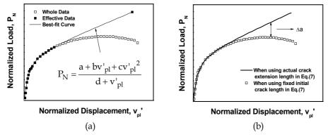
Fig. 7. J-R curve estimation concept on normalization method (a) Optimal best-fit for effective data pair (b) Crack extension length estimation from normalized curve
