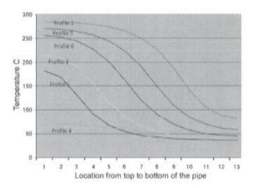
Fig. 5. Calculated Temperature input to the Approximate Numerical Model<sup>[4]</sup>
