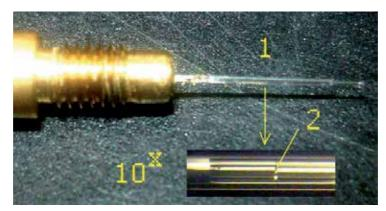
Fig. 19. General view of FFPI-based pressure sensor 1 – sensing element; 2 – FFPI cavity with  $\Delta G$  length (10<sup>x</sup> magnifying)
