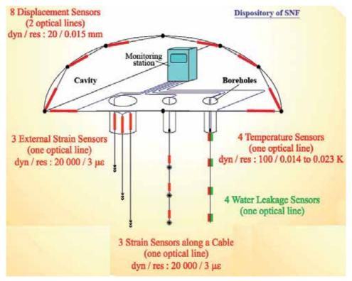
Fig. 22. Configuration of the OFS system in SNF repository
