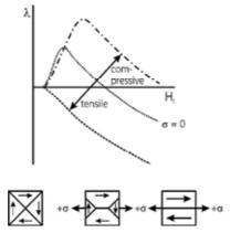
Fig. 4. Lengthwise magnetostriction and influence of mechanical stress
