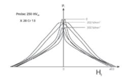
Fig. 10. Incremental permeability profile curves documenting the influence of mechanical stress, steel quality X20Cr13
