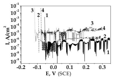
Fig. 9. PD curves of HAS in MCM with 1 mg/L Cl-, 1 mg/L SO4^2-, 5  $\mu$ g/L Cu\_{total} and 2 mg/L MEA:
