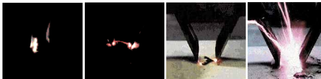
(a) Scintillation discharge (b) Arc discharge (c) Discharge and carbonization (d) Intense discharge Fig. 8. Example of discharge events with 100 kGy irradiated M-PC.
