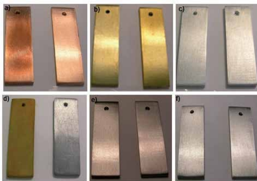
Figure 13. Appearance of samples after corrosion tests for diesel fuel containing up to 7% FAME after 6 months of storage: a) copper, b) brass c) aluminum, d) lead, e) C45 steel and f) S235JR steel (left: sample exposed to liquid, right: – after exposure in vapors)
