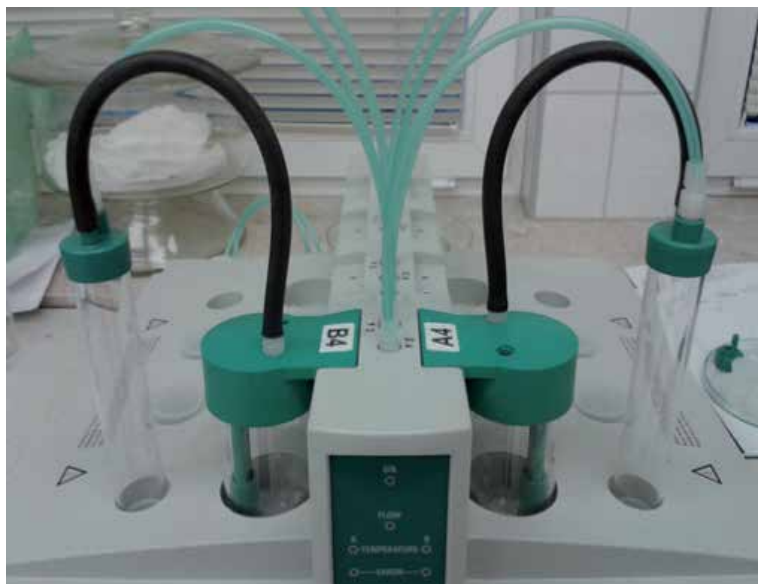
Figure 31. A test assembly for oxidation stability tests according to EN 15751 (Rancimat method).
