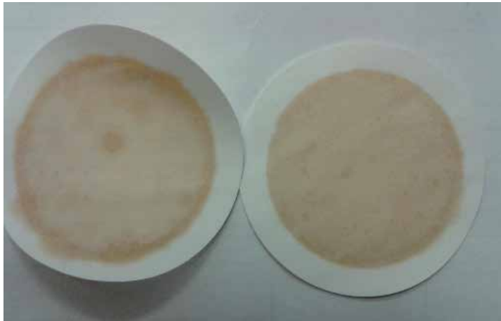
Figure 29. Insolubles, formed by oxidation during storage of diesel fuel with 7% (V/V) of a biocomponent.
