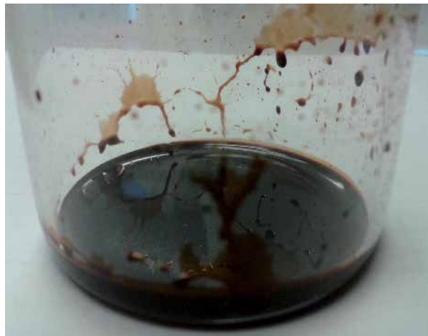
Figure 30. Solubles (gums), formed by oxidation during storage of diesel fuel with 7% (V/V) of a biocomponent.
