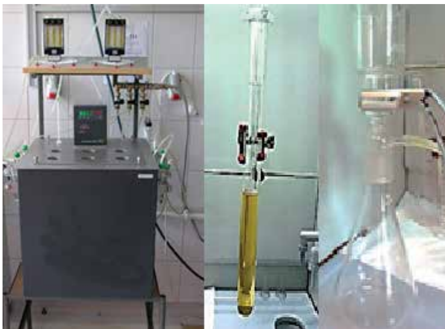
Figure 27. A test assembly for oxidation-stability tests of diesel fuels according to the standard EN 12205.
