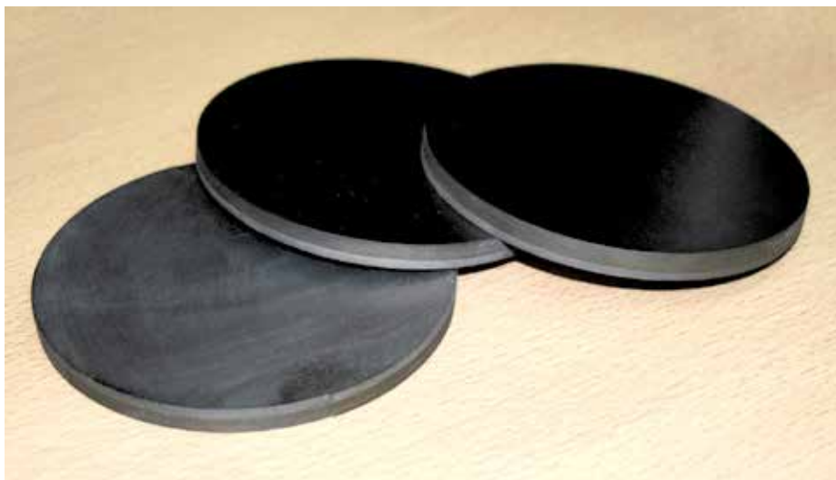
Fig. 4. Disc targets based on titanium carbonitride, titanium silicide, and titanium aluminide.
