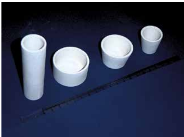
Fig. 9. AlN crucibles obtained by slip casting with an aqueous suspension containing 50-vol.% solids.
