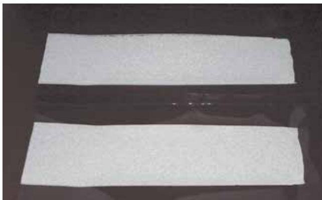
Fig. 12. Green tapes obtained by tape casting from the aqueous AlN-based suspensions.
