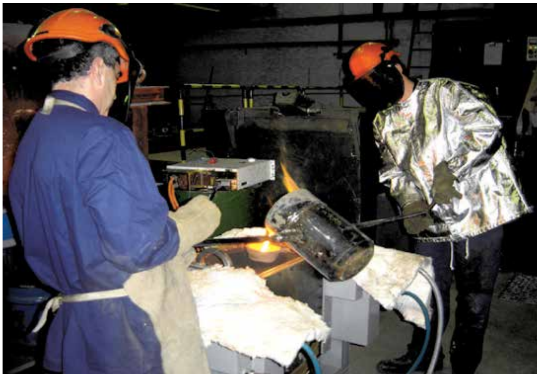
Fig. 12. Mould filling with steel+carbides
