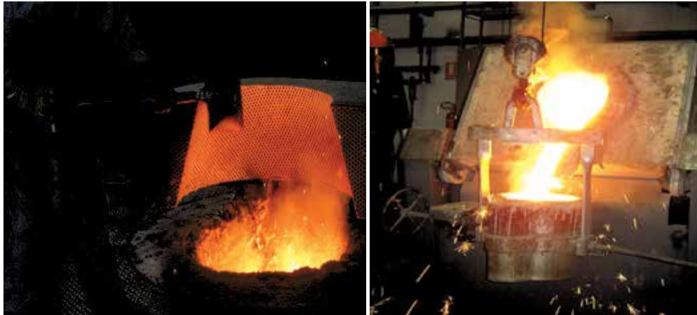
Fig. 11. Masteralloy addition and pouring of steel+carbides
