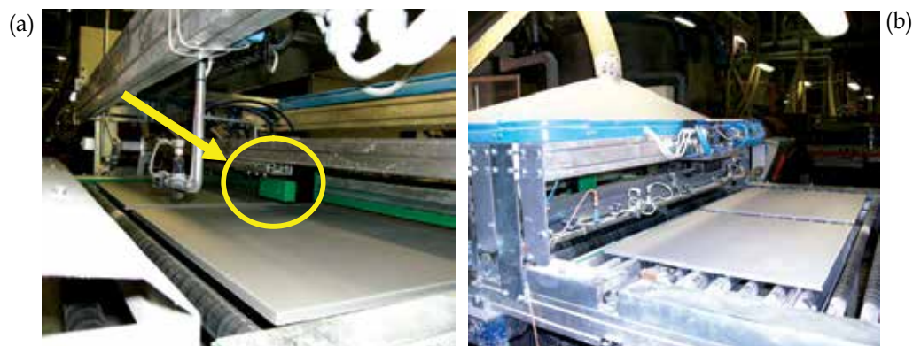
Fig. 8. (a) Head with the sensor holder; (b) Support for on-line positioning
