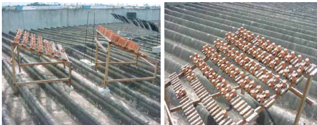
Fig. 11. Samples on terrace exposed on the roof directed to the best insulation direction according to the local coordinates
