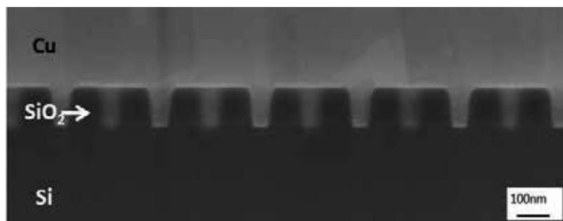
Figure 15. Cross-sectional SEM images of Cu filled into nanoscale vias (60 nm diameter, 120 nm depth) by ED-SCS with the continuous-flow reaction system with current density 2.83 \text{ A/dm}^2 of applied direct current.
