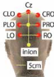
Fig. 9. Electrode positions. Three pairs of electrodes over the occipital (LO and RO), parietal (PLO and PRO), and central (CLO and CRO) regions were used to construct three channels of bipolar derivation. LO, PLO, and CLO were connected to the plus input, and RO, PRO, and CRO were connected to the minus input. A ground electrode was applied over Cz.
