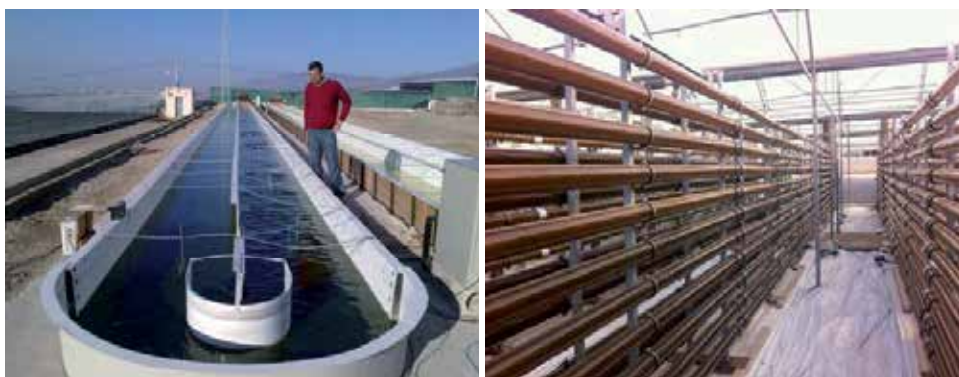
Figure 17. Microalgae culture in open system (raceway) and close photobioreactor (Almeria University and Palmerillas Research Center).
