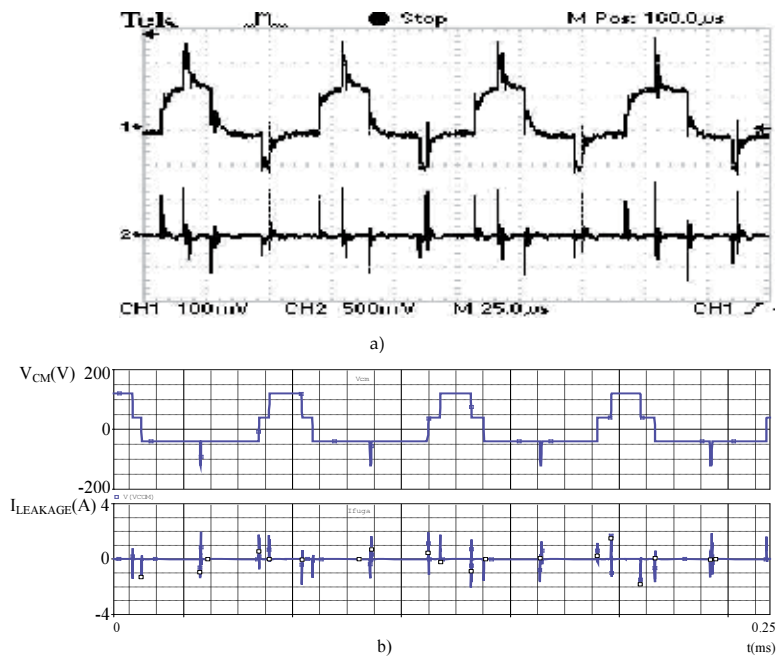
Figure 27. V_{CM} – CH 1, I_{LEAKAGE} – CH 2 - a) measured, b) simulated - (IM1hp2)
