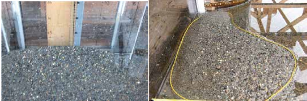
Figure 5. Scour pattern with nonuniform sand from Case 1
