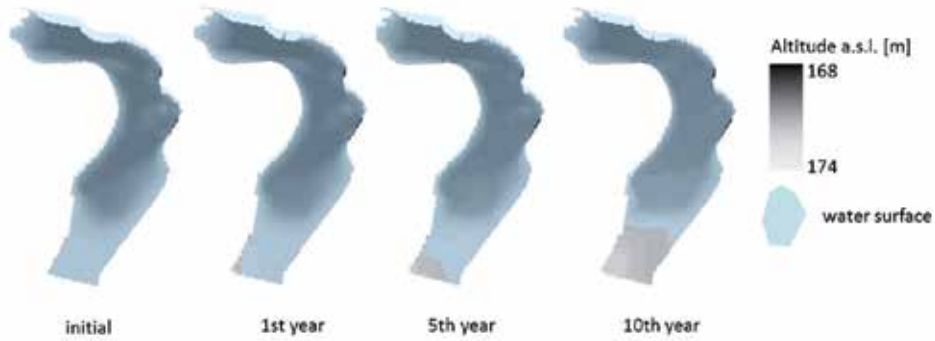
Figure 13. Siltation of the Baderitz Reservoir.
