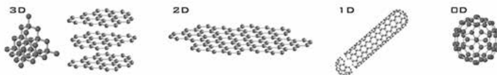
Fig. 1. Crystal structures of different allotropes of carbon. (Left to right) Three-dimensional diamond and graphite (3D); two-dimensional graphene (2D); one-dimensional nanotubes (1D); and zero-dimensional buckyballs (0D) (Mikhail & Katsnelson, 2007).
