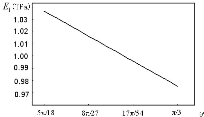
Fig. 12. Elastic modulus of the equivalent model of graphene along the 0^\circ fiber
