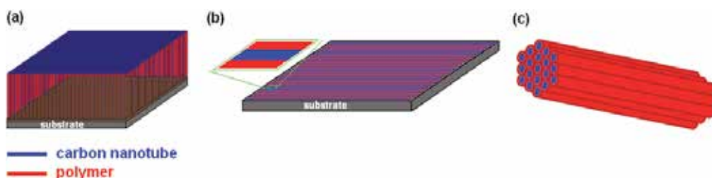
Fig. 9. Schematic illustration of the aligned nanotube/polymer composites in the forms of (a) array, (b) film, and (c) fiber.
