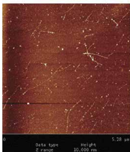
Fig. 10. AFM height image of electric arc SWNTs deposited on mica from solution after debundling process of ternary intercalation compounds prepared by a liquid medium intercalation method. Height measurements show a height of about 1 nm on all nanotubes measured consistent with the presence of isolated SWNTs in the solution. From (Pénicaud et al., 2005) Copyright 2005 by the American Chemical Society.
