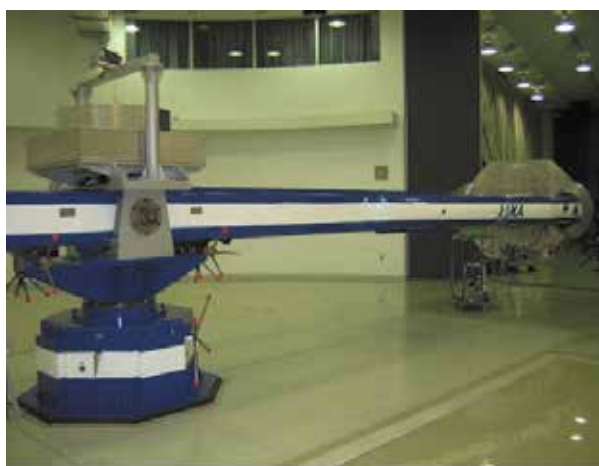
Fig. 12. Photograph of the rotation acceleration generator of JAXA.
