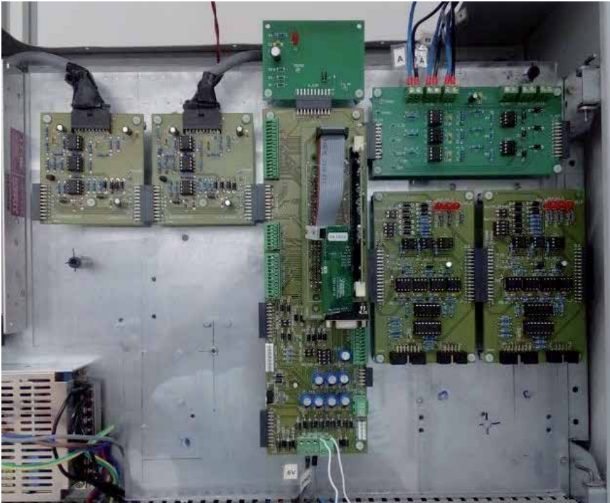
Figure 13. Modular electronic control unit printed circuit boards.
