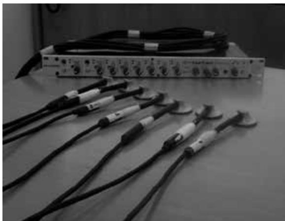
Figure 2. Multi-channel equipment for computerised respiratory sound analysis.
