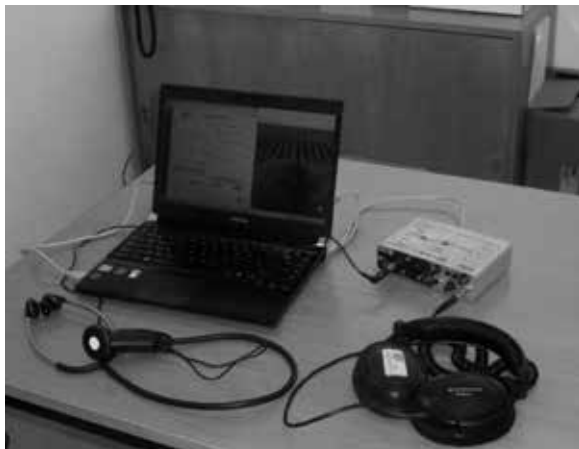
Figure 1. Single-channel equipment for computerised respiratory sound analysis.
