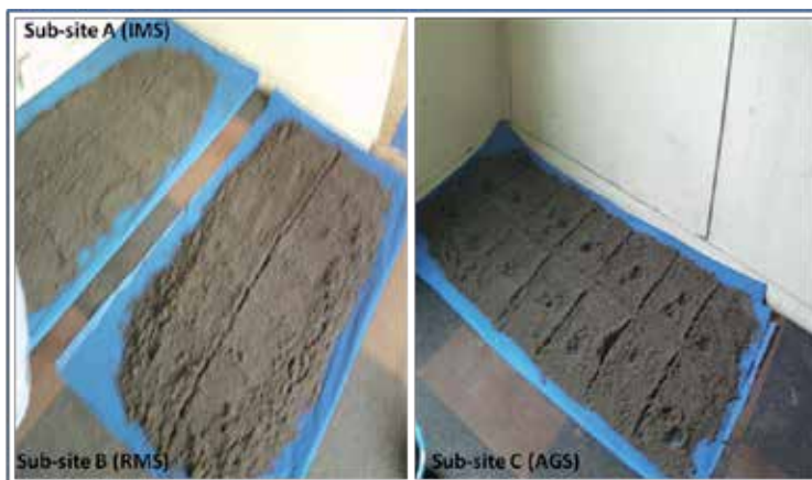
Figure 5. The three different sample bulks showing grid template of 12 cells created on each sample, from which samples were collected for physicochemical analyses
