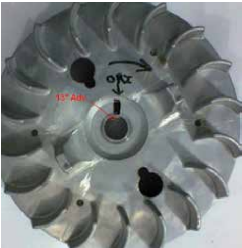
Figure 4. Flywheel with mark indicating new keyway providing spark advance.
