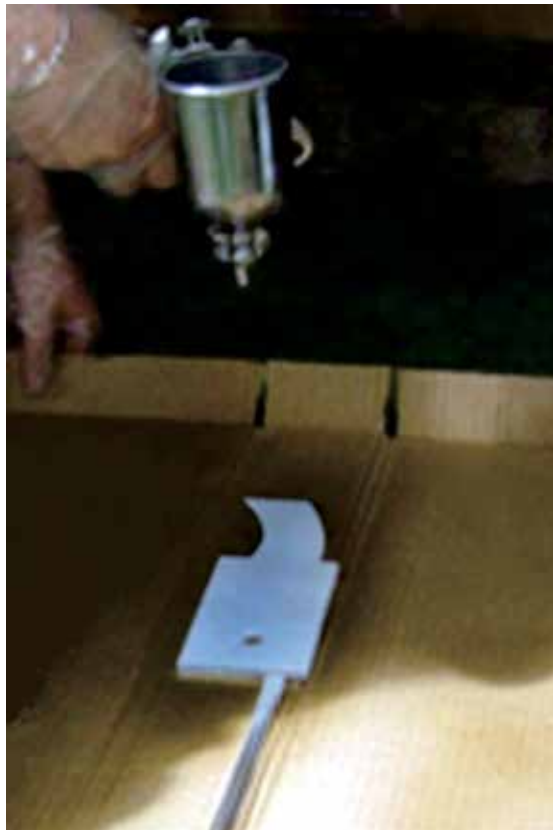
Figure 4. Spraying the paint on the surface.
