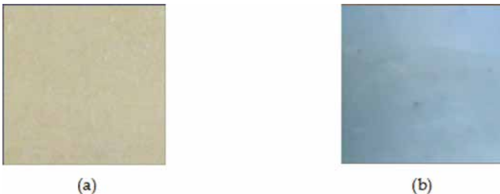
Figure 5. Surface coated with PSP. (a) Paint from ISSI; (b) paint from ICAS.
