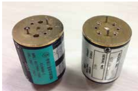
Figure 3. One popular type of waveguide thermistor mount.
