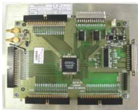
Figure 6. One FPGA programmable logic module architecture.
