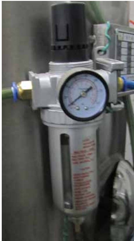
Figure 7. Oil and water filtering regulator for spraying air brush.
