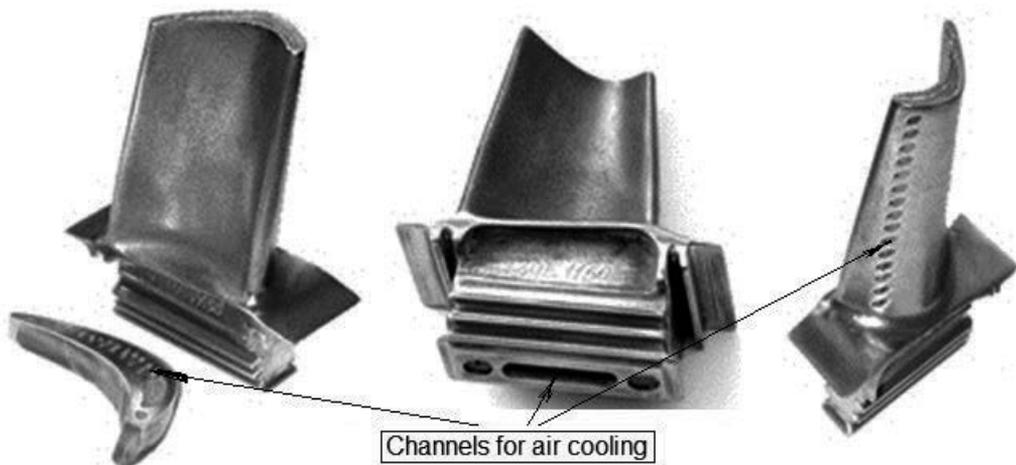
**Figure 1.** Air-cooled and thermal barrier-coated high-temperature turbine blade for turbojet engine Al31-F.
