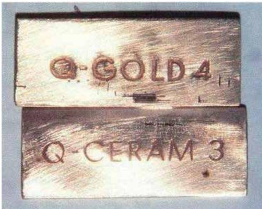
**Figure 8.** The corrosion test samples are two plates of noble alloy connected by soldering
