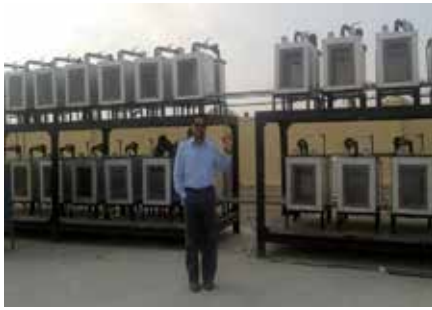
a- Double deck MSF desalination test pilot unit
